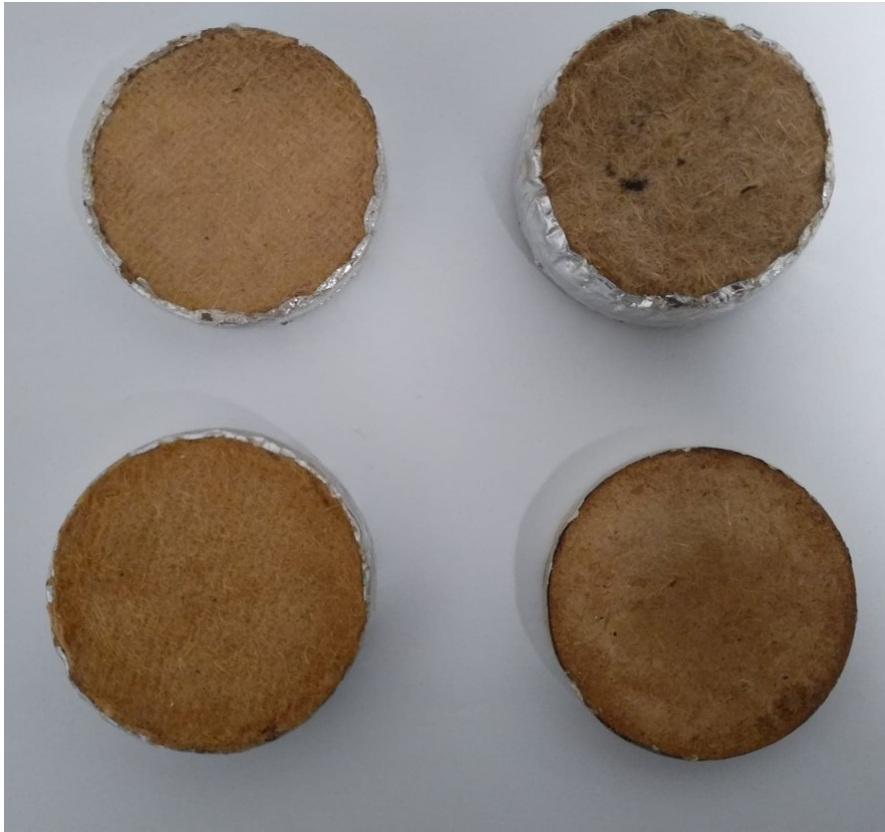
Figure 2: Photograph of the samples: From left to right and top to bottom: LDF ( 255 \text{ kg} \cdot \text{m}^{-3} ; 10 mm), LDF ( 145 \text{ kg} \cdot \text{m}^{-3} ; 20 mm), LDF ( 234 \text{ kg} \cdot \text{m}^{-3} ; 19 mm), and MDF ( 655 \text{ kg} \cdot \text{m}^{-3} ; 10 mm)
