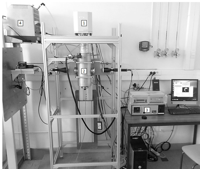
Figure 4: Experimental setup, showing 1: magnetic suspension balance, 2: heating jacket enclosing the measuring chamber, 3: humidity generator, and 4: cryothermostat for temperature control
