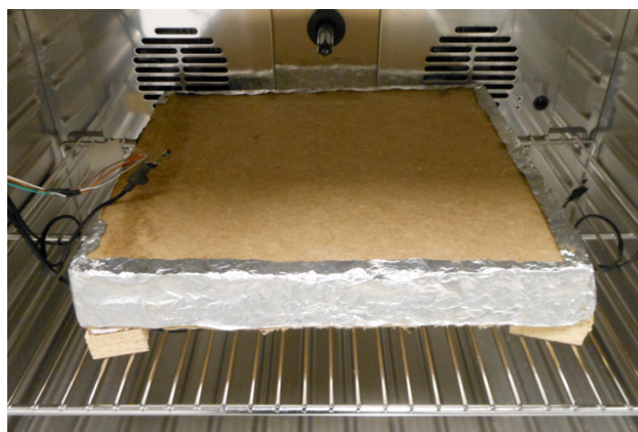
Figure 1: Schematic cross-sectional view of the double plate (top) and photograph of the sample placed inside the climatic chamber (bottom).
