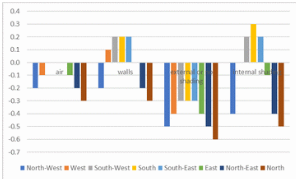
Figure 56: Mean bias error of the temperature (°C) depending on the building orientation.
