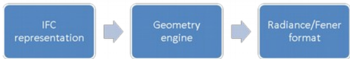
Figure 16: Simplified workflow of geometry processing from IFC.
