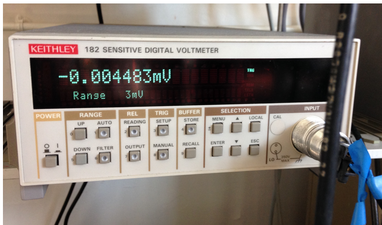
FIGURE 2.16 – NanoVoltmètre KEITHLEY ® 182 sensitive digital voltmeter
