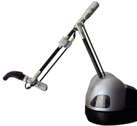
Figure 4.4: The Virtuose 6D haptic device
