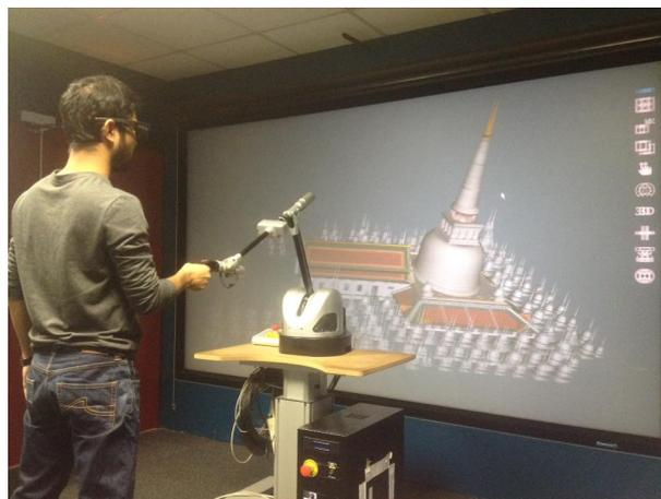
Figure 4.2: The stereoscopic display with shutter glass
