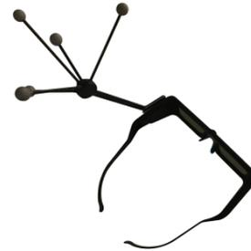
Figure 4.3: MIHRIAD miniCAVE and a shutter glasses with tracking markers
