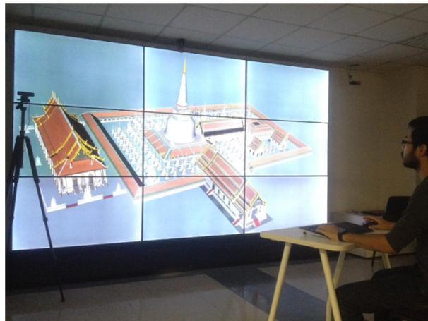
Figure 4.1: The Powerwall with 3x3 tiled displays
