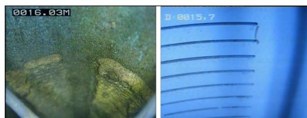
**Figure 4** Video inspection of the injection wells of HA doublet (Left: Clogged well screens, Right: Initial)
