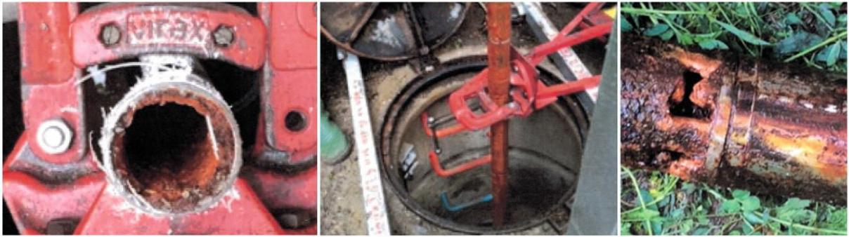
**Figure SI.1.** Deposits on the well pump and on the inner surface of the pumping-well column
