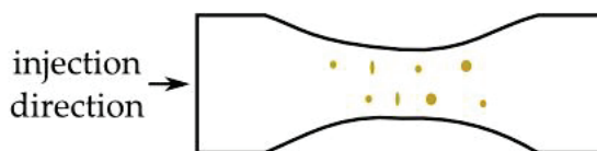
Figure 11 Schematic representation of the initial cavities observed in the sample in the case of \theta = 0^\circ before tensile experiment
