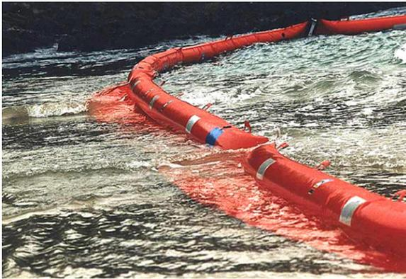
Fig. 1. Boom behaviour under a strong current.
