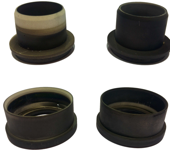
Figure 4.16: Ceramic walls of the ISCT200-US (left) and ISCT200-MS (right) highlighting, for the MS case, the absence of the characteristic erosion pattern in the black deposit formed on the walls.
