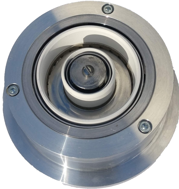
Figure 6.4: The ISCT200-MS-V2 magnetically shielded, low power, permanent magnet Hall thruster
