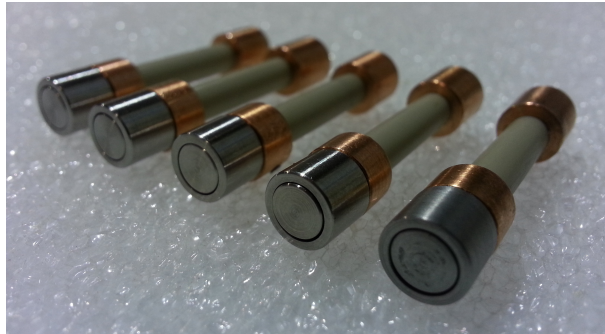
Figure 2.3: Planar probes with their guard ring as used in the NExET vacuum chamber
