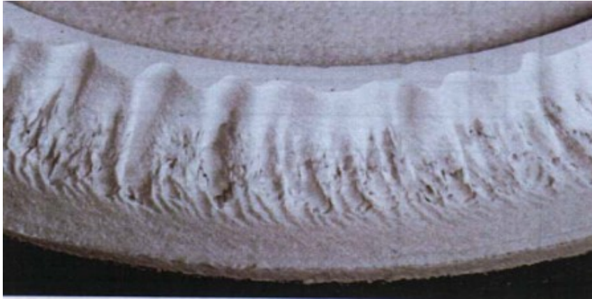
Figure 4.4: Anomalous erosion as seen on the PPS-1350 thruster after 3500 hours of operation [2]
