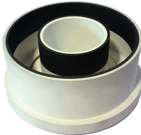
Figure 5.1: Discharge channel with the graphite inserts. The graphite inserts cover two thirds of the discharge channel length.
