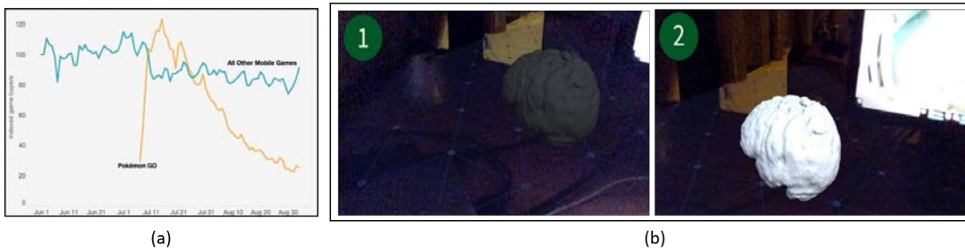
Figure 1.3 – (a) The image represents the impact of PokémonGO compared to previously existing gaming applications. (b) The images show an augmented scene (virtual white object) using ARCore. The synthetic object fits the overall brightness with the capture of the scene. Nonetheless, it is still distinguishable from the real environment.
