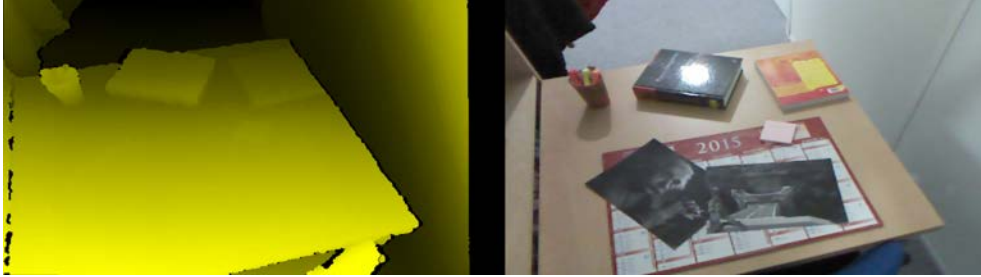
Figure 4.6 – RGB-D capture of the scene using the Kinect v1 sensor: the left image shows the input depth map. The right image shows the input color image.
