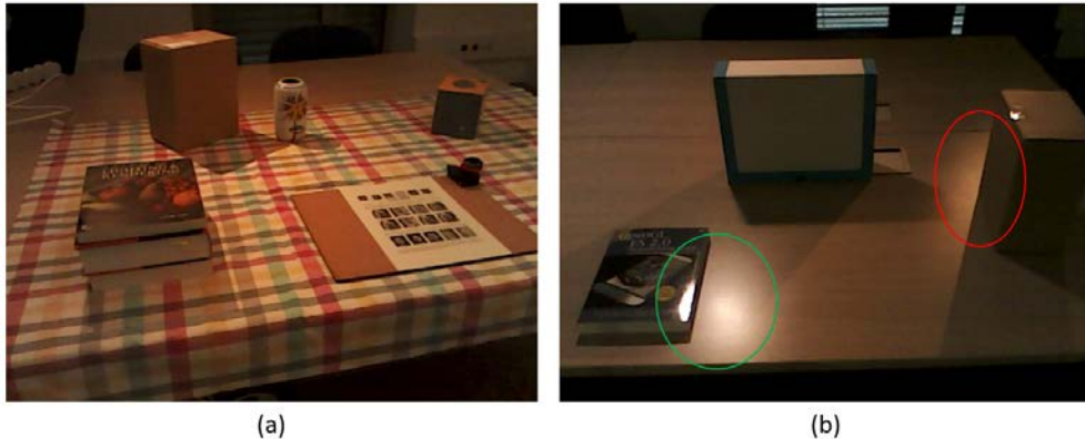
Figure 5.1 – Critical scenarios for the method described in chapter 4. (a) Capture of a real scene where most surfaces hold only a Lambertian property. (b) Capture of a real scene with two main light sources: the specular effect created by the first light source is captured (green-circled) whereas the second one is mostly occluded by the brown box (red-circled).
