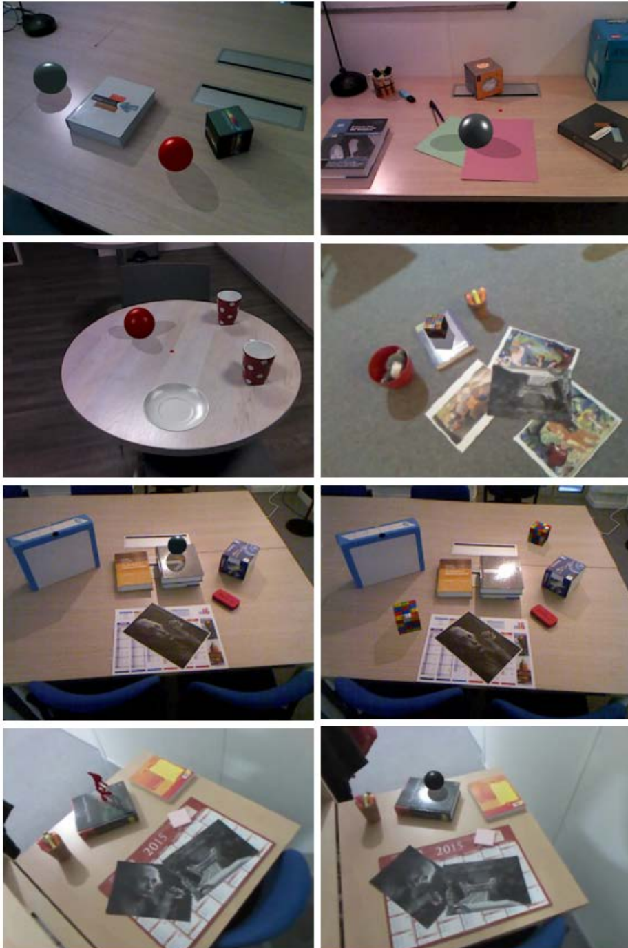
Figure 4.21 – Augmented scenes, with different reflectance and illumination conditions. We demonstrate correctly rendered virtual objects as they occlude real specular reflections (note the presence of the recovered diffuse component in the occluded region) and cast realistic shadows on real surfaces.
