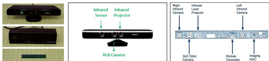
Figure 2.4 – Examples of 3D sensors: (left) Microsoft Kinect v1, Kinect v2 and R200 are represented row-wise (scaled) (center) Main components of the Kinect v1 (right) Main components of Intel R200 sensor.
