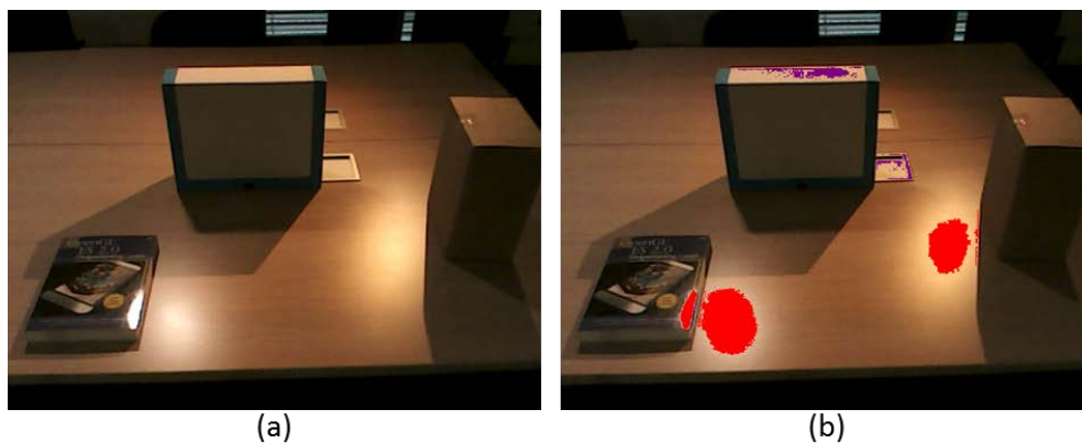
Figure 6.9 – (a) Input color image of the scene with two specular effects. (b) Detection of specular reflections: red pixels correspond to the detected specularities after discarding (magenta) pixels that do not check equation 6.9.
