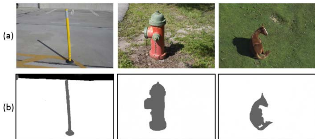
Figure 7.11 – (a) Images from available benchmarks [Zhu et al., 2010][Vicente et al., 2016]. (b) Manually crafted segmentation map for images in (a).
