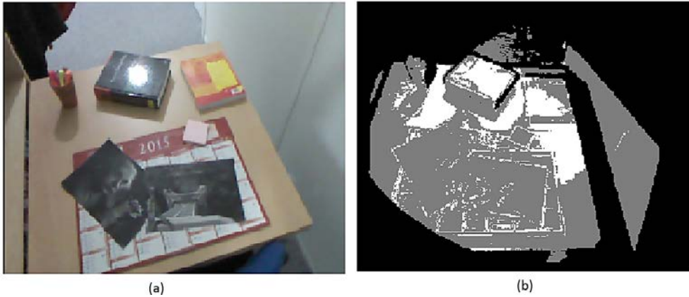
Figure 4.11 – (a): color image of the scene. (b): Luminance Profile based classification: the black pixels represent the discarded points (mostly occluded within the sequence), the grey ones correspond to constant luminance profiles and the white ones hold variable luminance profiles.
