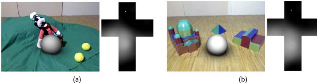
Figure 3.12 – Augmented real scenes (a) and (b) with a virtual grey sphere (left) and their recovered illumination (right). Figures from [Gruber et al., 2012].
