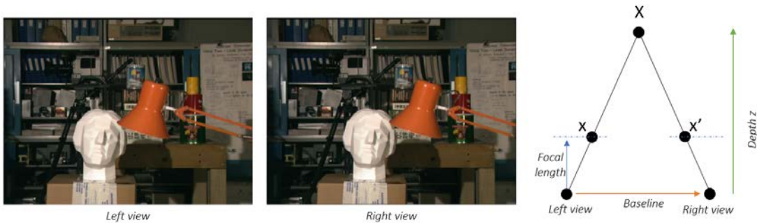
Figure 2.2 – First and second columns are views of a stereo pair. Third column is an outline of the operation of a simple stereo rig using stereo images to recover the 3D structure of the scene.
