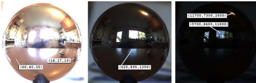
Figure 3.4 – Three photographs of a mirrored ball (chrome sphere) used to recover a high dynamic range of a light probe image. Figures from [Debevec, 1998].
