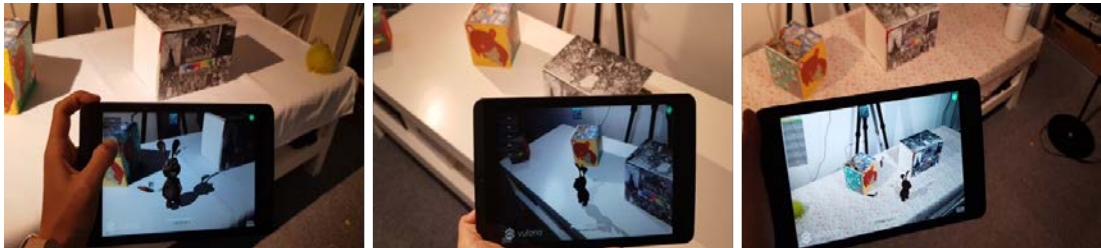
Figure A.1 – Captures of our Mixed Reality (MR) application for real scenes with a uniform and Lambertian surface (left), a uniform and specular surface (center) and a challenging textured surface (right). The lighting condition can be changed within the MR experience.
