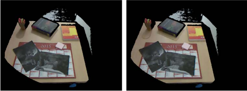
Figure 4.16 – Refined diffuse component. The left image is the diffuse component estimate. The right image demonstrates the results of our diffuse recovery for occluded points. Because the area light source was approximated by a point light source, we can observe that the edges of the soft shadows were not correctly recovered.
