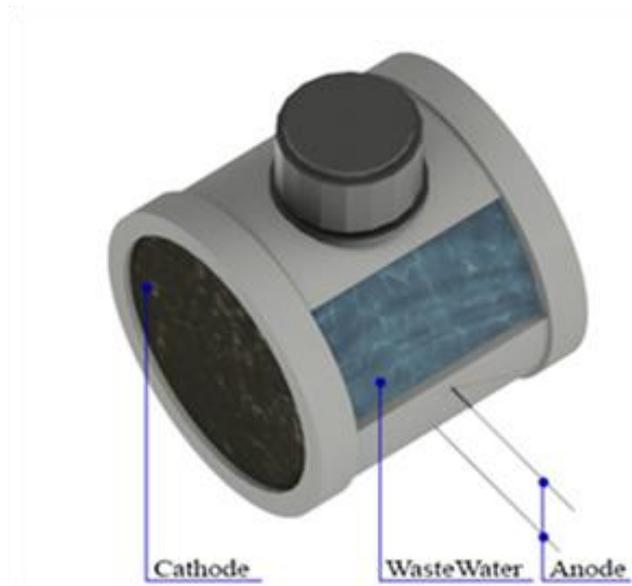
*Fig. 2.14: 3D graphical section of a lab-scale WWMFC*
