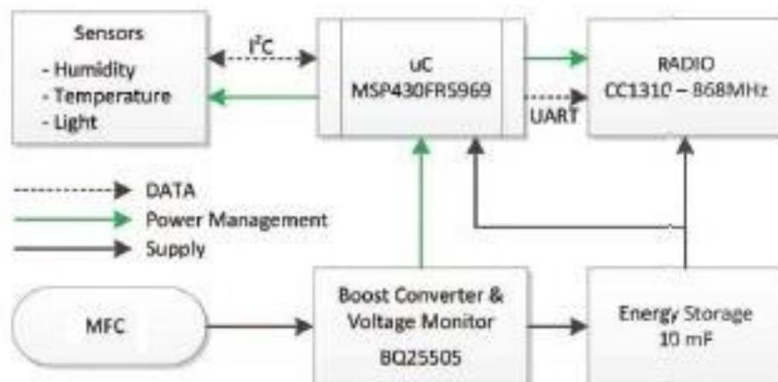
Fig 5.13: Block diagram for a long range WSN powered by MFC [112]
