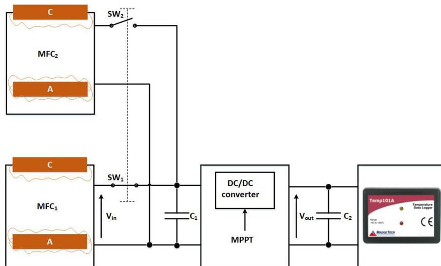
Fig. 5.16: Power management system for Continuous mode supply with 2 MFCs [56]
