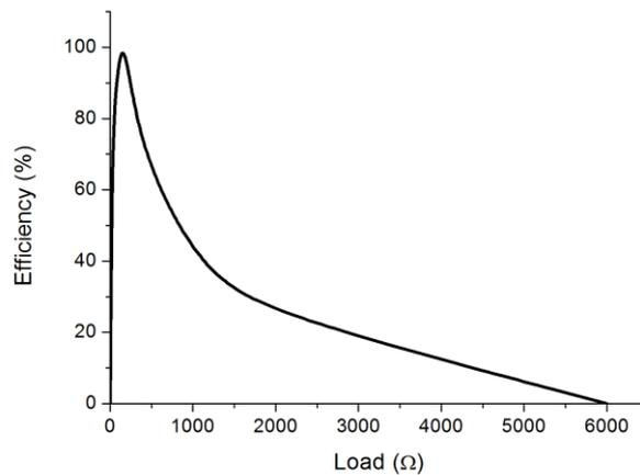
Fig. 2.17: Typical effect of load on MFC efficiency[29]
