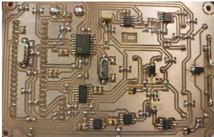
*Fig. 3.1: Photo of the top layer of the Measuring Board*
