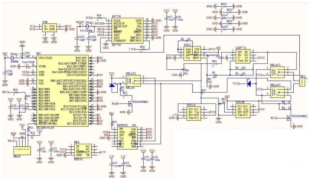
Fig. 3.3: Schematics of the custom measuring instrument
