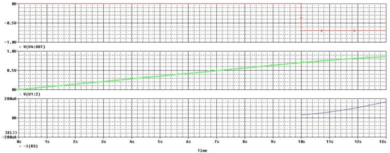
Fig. 5.10: Results of the simulation of the proposed feedback control loop
