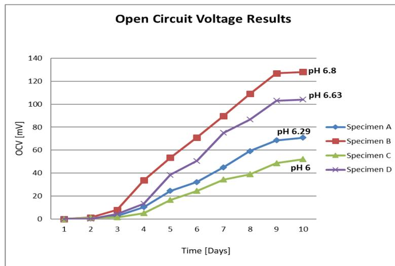
Fig 4.4: Open Circuit Potential evolution chart results.
