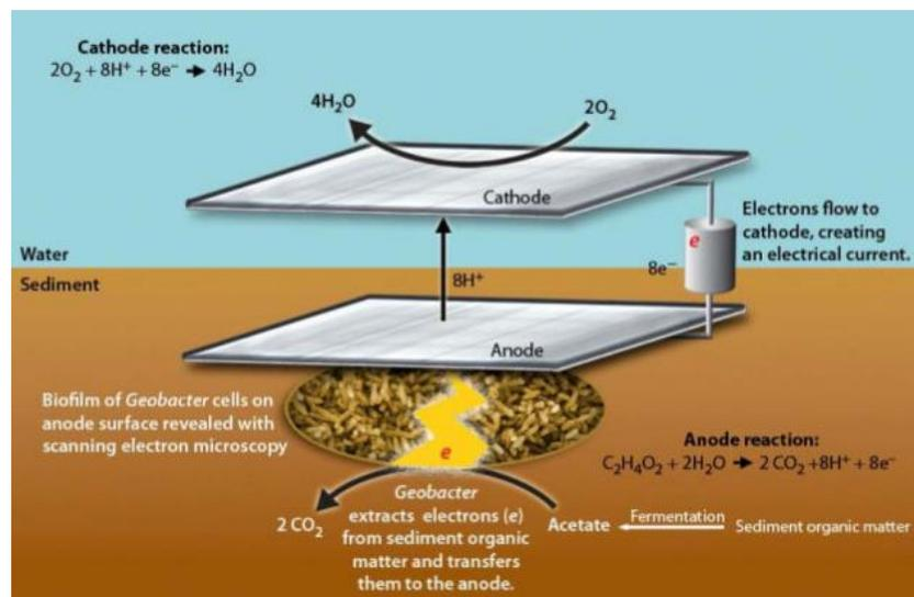
Fig 2.4: Typical operation of a Benthic Microbial Fuel cell [9]
