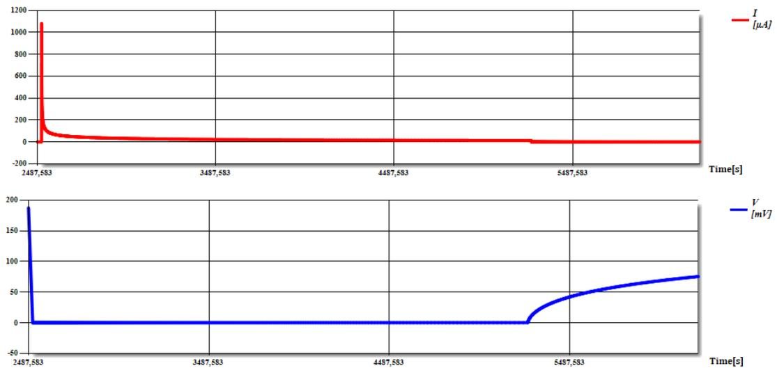
Fig 4.9: The discharge phase of a single WWMFC
