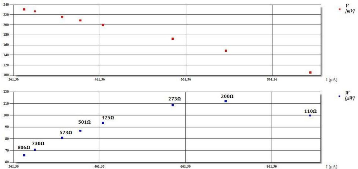
Fig 4.18: WMMFCs in parallel configuration power chart
