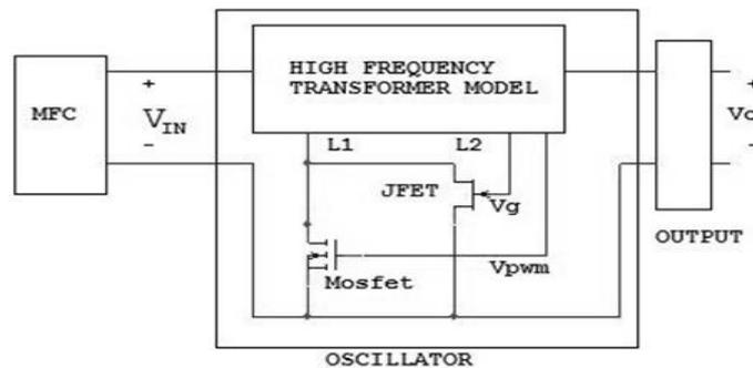
Fig. 5.1: Converter scheme: configuration with a transformer.
