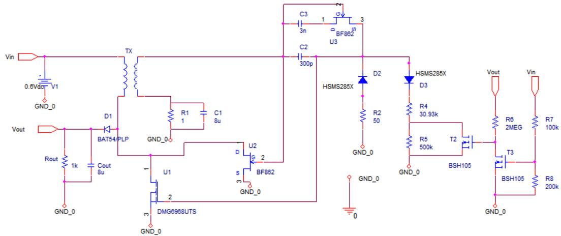
Fig 5.4: OrCAD schematic of the adapted circuit for TMFC
