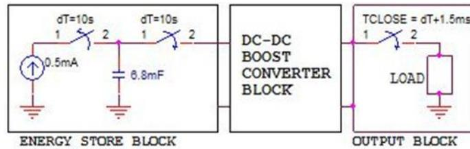
Fig 5.6: Block diagram of the proposed system with TPS61221 inside converter block
