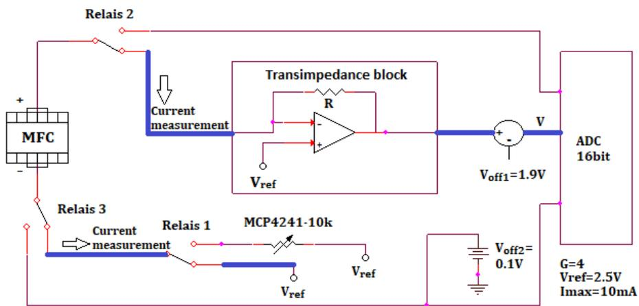
Fig. 3.6: Current measurement Block Diagram
