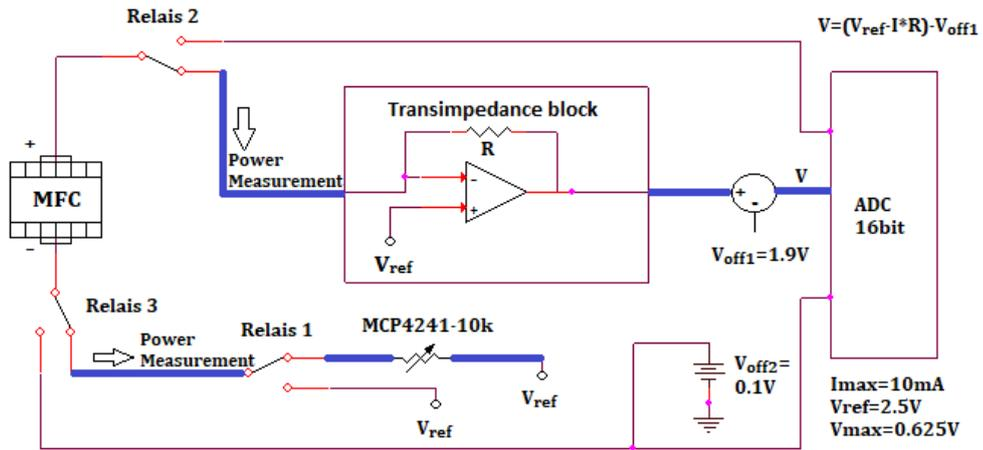
Fig. 3.7: Power measurement Block Diagram
