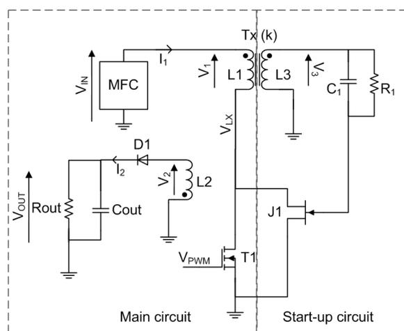
Fig. 5.11a: Simplified circuit of the flyback converter
