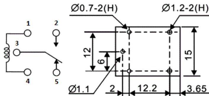
Fig. 7.4: Output configuration of a LEG-5 RELAYS by RAYEX ELEC
