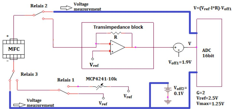
Fig. 3.5: Voltage measurement Block Diagram
