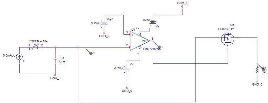
Fig 5.9: Scheme block of the feedback control loop
