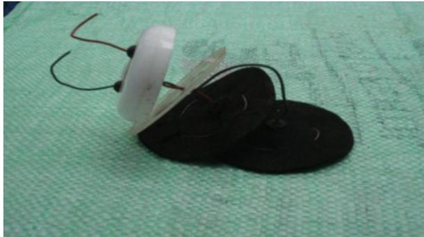
*Fig. 2.9: Photo of the electrodes used for lab-scale TMFC made of carbon felt*
