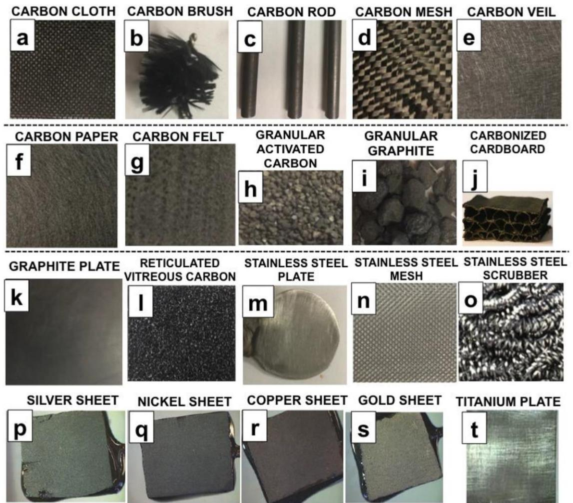
Fig. 2.7: Digital photographs of carbon cloth (a), carbon brush (b), carbon rod (c), carbon mesh (d), carbon veil (e), carbon paper (f), carbon felt (g), granular activated carbon (h), granular graphite (i), carbonized cardboard (j), graphite plate (k), reticulated vitreous carbon (l), stainless steel plate (m), stainless steel mesh (n), stainless steel scrubber (o), silver sheet (p), nickel sheet (q), copper sheet (r), gold sheet (s), titanium plate (t) (Santoro et al. [114]).
