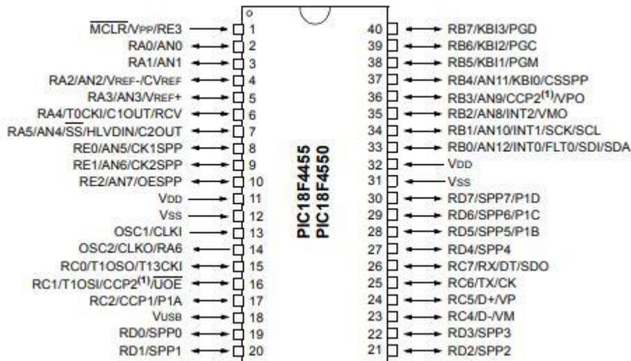
Fig. 7.7: Pin configurations of PIC18F4550 40-pin PDIP package
