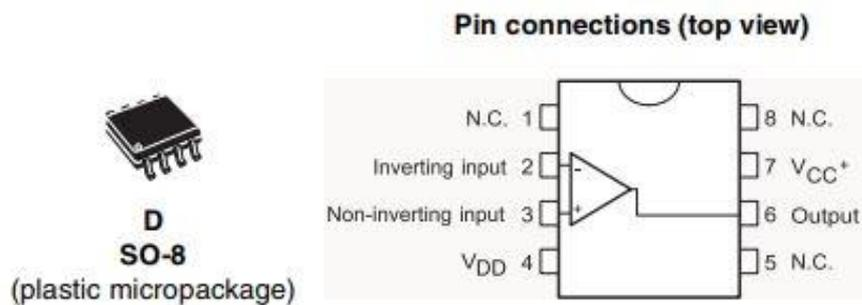
Fig. 7.6: TS921 SOIC\_8 package and pin configuration
