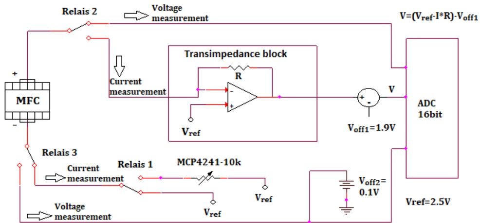
Fig. 3.4: Block Diagram of the custom measuring instrument
