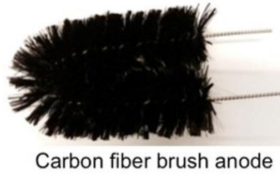
Fig. 2.11: Photo of carbon fiber brush anode
