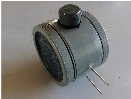
Fig. 2.15: Photo of a lab-scale WWMFC
