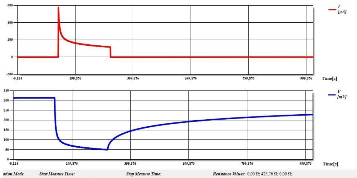
Fig 4.25 Results in term of voltage and current delivered during time (3 minutes measurement time) for a WWMFC before polarization method applied
