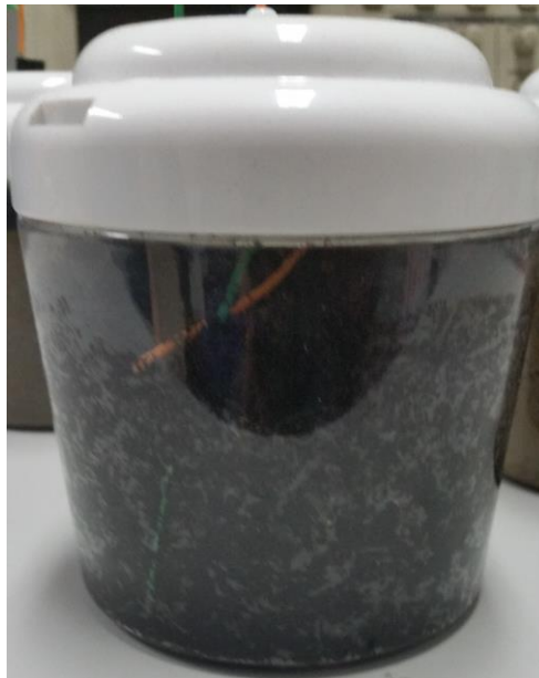
Fig. 2.9: Photo of the electrodes used for lab-scale TMFC made of carbon felt
