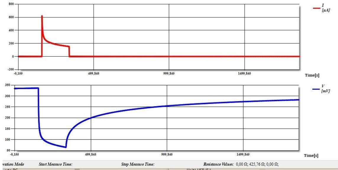
Fig 4.24: Results in term of voltage and current delivered during time (3 minutes measurement time) for a WWMFC after polarization method applied
