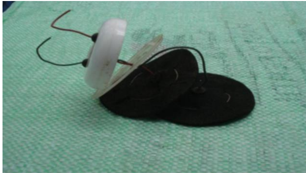
Fig. 2.9: Photo of the electrodes used for lab-scale TMFC made of carbon felt
