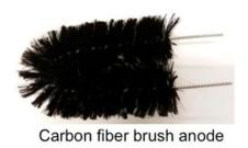
Fig. 2.11: Photo of carbon fiber brush anode
