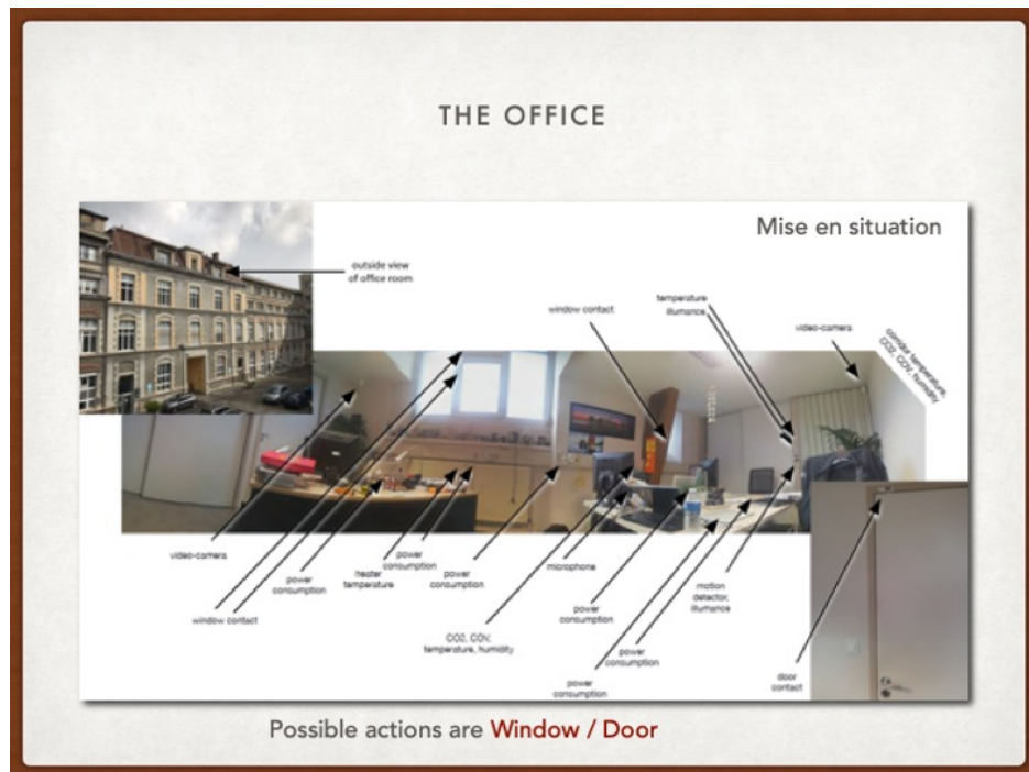
Figure 6.11: office and sensors
