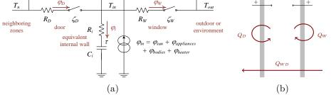
Figure 4.2: Building simulation models: (a) thermal model [106], (b) aeraulic model [74]
