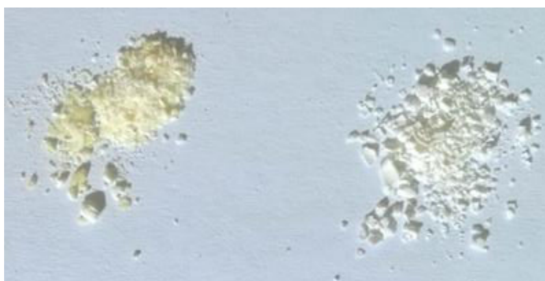
Figure IV. 8. Picture of \alpha -alkynyl, \omega -dodecyltrithiocarbonate PNIPAM before (left) and after (right) removal of the trithiocarbonate chain-end group using AIBN as radical initiator in 1,4-dioxane at 80°C.
