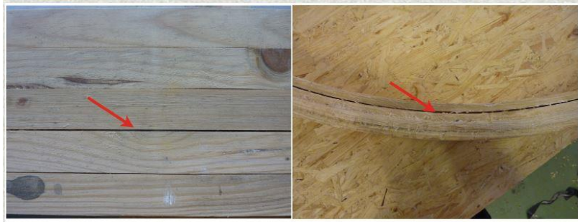
Figure 1-2: Detachment of the adhesive interface [7].
