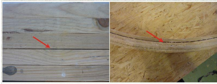
Figure 1-2: Detachment of the adhesive interface [7].
