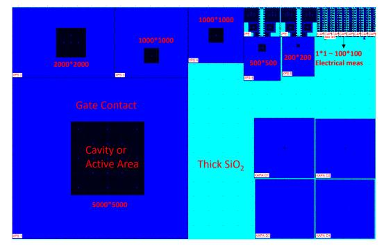
Figure 6.7: Top view of the test structures with various device sizes, used for XPS and electrical measurements
