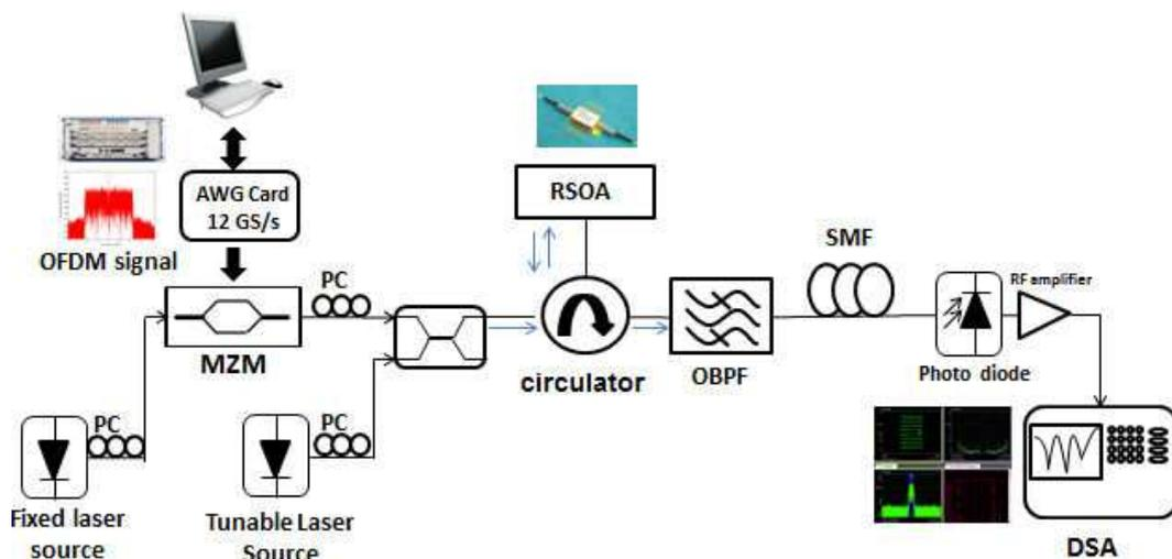
Figure 3- 34 : Experimental setup of the OFDM wavelength conversion.
