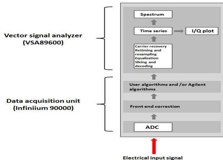
Figure 3- 6 : block diagram of the digital signal analyzer used (document from Agilent technologies)
