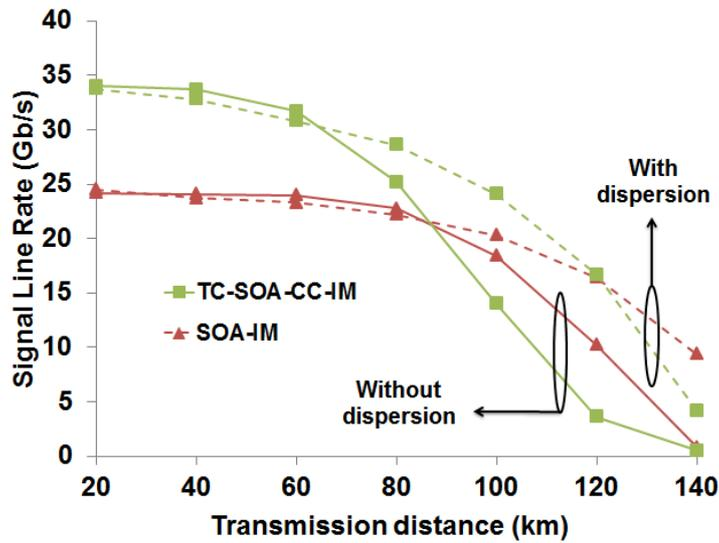
Figure 4- 32 : Signal line rate versus reach performance for the cases of including and excluding the CD.
