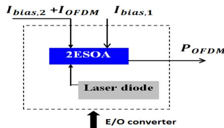
Figure 4- 19 : 2E-SOA E/O converter configuration
