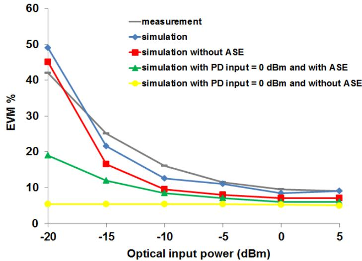
Figure 3- 15 : EVM vs Input power for 2GHz OFDM-16 QAM, the bias current is 65 mA, the wavelength is 1560 nm. (PD: photodetector).
