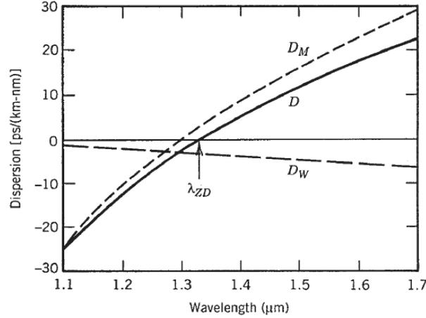
Figure 1- 19 : Dispersion spectrum of a conventional single-mode silica fiber. The total dispersion  $D$  and the relative contributions of the material dispersion  $D_M$  and of the waveguide dispersion  $D_W$  are also shown [1].
