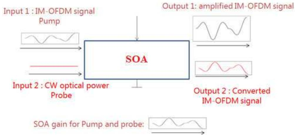
Figure 3- 32 : Principle of XGM wavelength conversion in an SOA.
