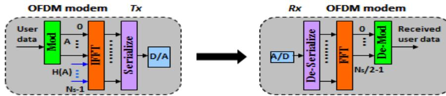
Figure 1- 24: OFDM electrical back to back simulation setup.
