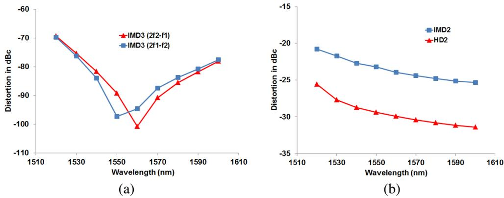
Figure 2- 20: Distortion simulation dBc values for (a) IMD3 signals (b) IMD2 and HD2, as function of wavelength for a 7 mA input AC current, Input power to the RSOA is -20 dBm, bias current is 65 mA.
