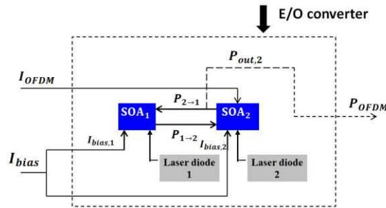
Figure 4- 23 : TC-SOA-CC E/O converter configuration
