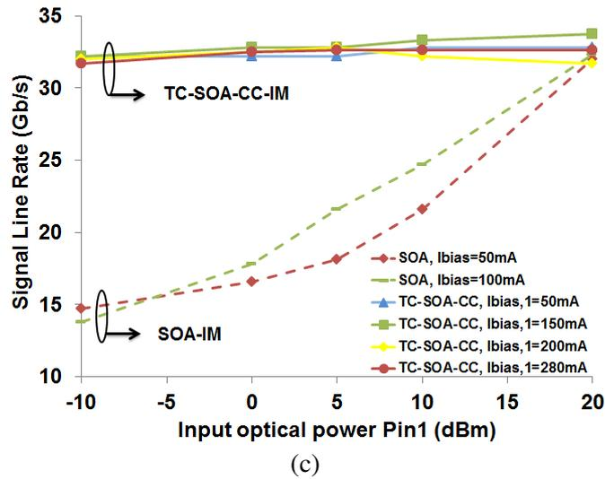
Figure 4- 29 : Signal line rate of TC-SOA-CC-IM and SOA-IM as a function of the input optical power  $P_{in,1}$ . (a)  $P_{in,2}=0dBm$ , (b)  $P_{in,2}=10dBm$ , (c)  $P_{in,2}=20dBm$ .
