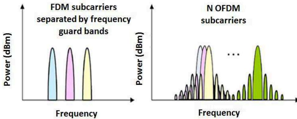
Figure 1- 8 : Spectra for FDM and OFDM.
