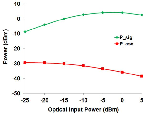
Figure 3- 14 : RSOA static characterisation of the output signal power and ASE signal power versus the RSOA input signal power.
