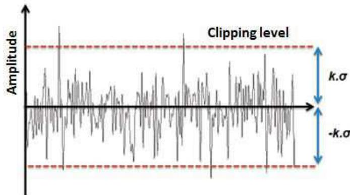
Figure 1- 9 : Arbitrary OFDM signal truncated between two clipping thresholds  $-k$  and  $k$  [18].
