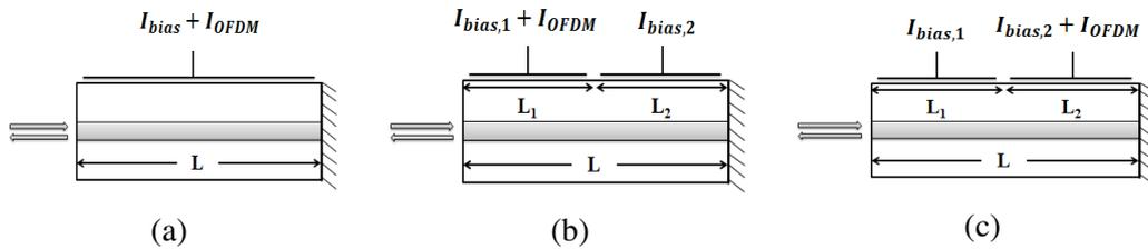
Figure 3- 28: Three studied RSOA configurations, (a) one electrode, (b) two electrodes with modulating the input section, (c) two electrodes with modulating the mirror section.
