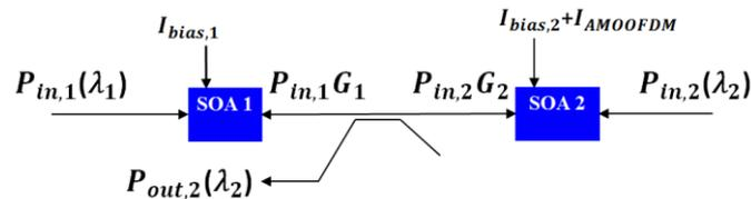
Figure 4- 24 : Schematic view of a TC-SOA-CC with contra propagating signals
