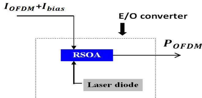
Figure 4- 5 : RSOA E/O converter configuration
