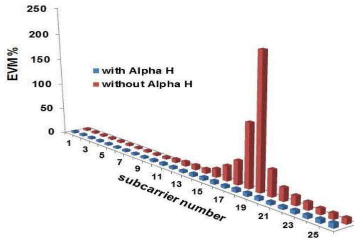
Figure 3- 20 : EVM per subcarrier in presence of 80 km fibre with  $\alpha_H = 0$  and with  $\alpha_H \neq 0$  for a 3 GHz OFDM-16 QAM signal, RSOA bias current is 65 mA, OFDM current is 7 mA, input power to RSOA is -15 dBm, wavelength is 1560 nm.(photodetector input = 0 dBm for all cases).
