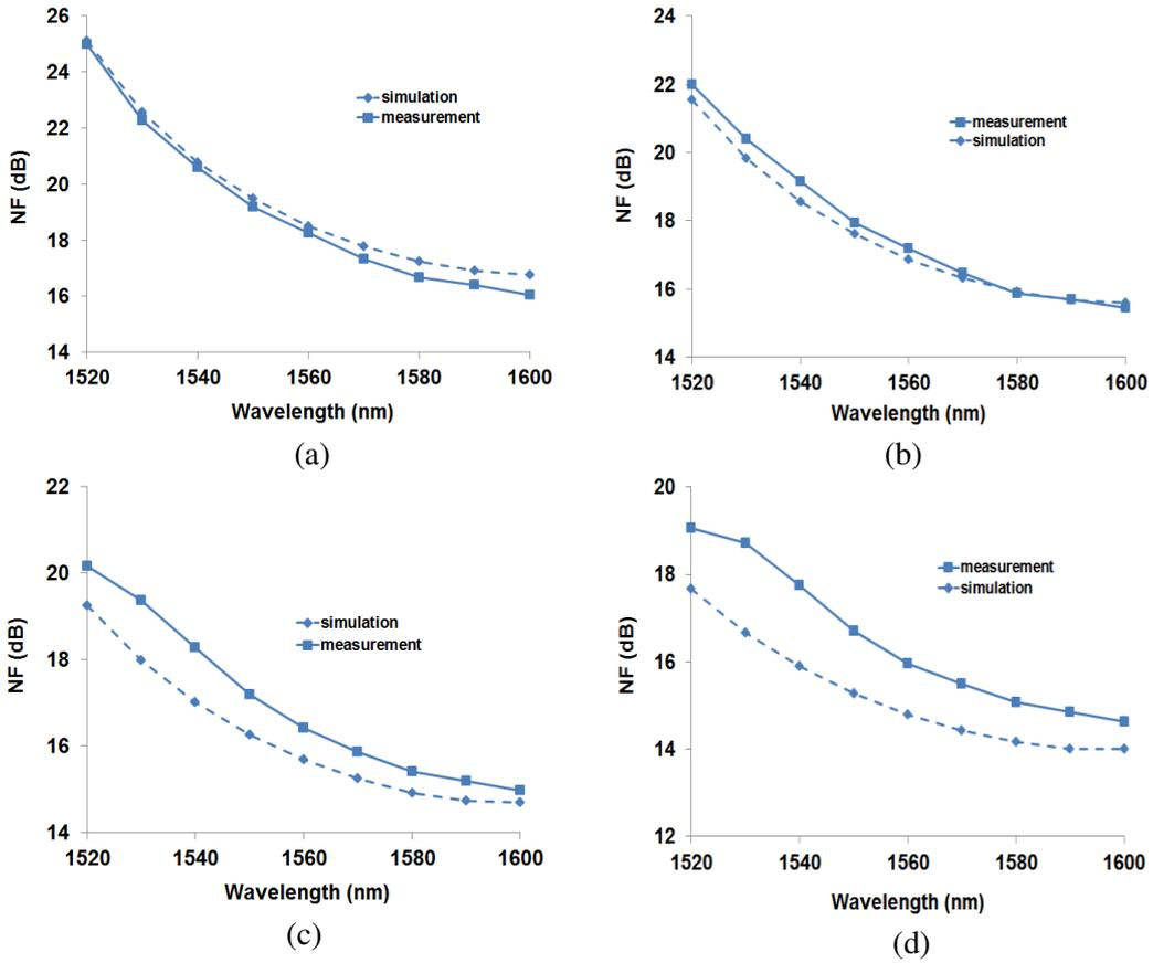
Figure 2- 7 : Measurements (dots) and simulated (solid lines) of the NF in function of the wavelength for an input power of 4dBm and a bias current of (a) 50 mA, (b) 60 mA (c) 70 mA, (d) 80 mA.
