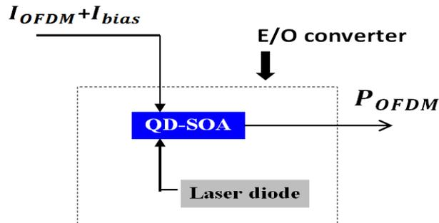
Figure 4- 7 : QD-SOA E/O converter configuration
