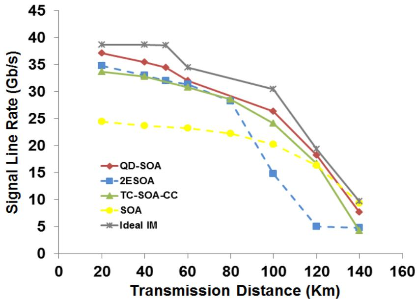
Figure 4- 33 : Signal line rate versus reach performance for five different IM configurations.
