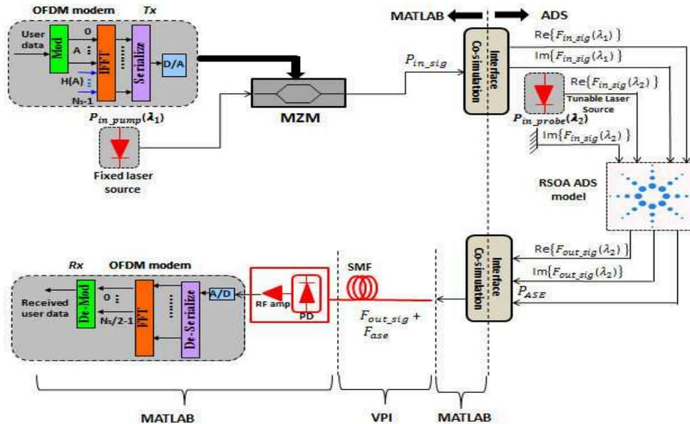
Figure 3- 33 : IM-OFDM wavelength conversion co-simulation platform using RSOA.
