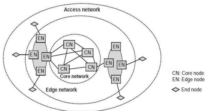
Figure 1- 5 : A typical optical networking architecture [18].
