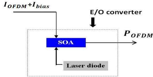
Figure 4- 3 : SOA E/O converter configuration
