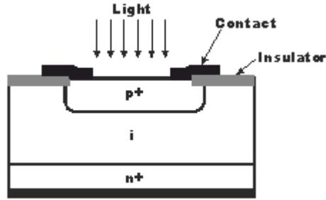
Figure 1- 21 : p-i-n photodiode structure [36]
