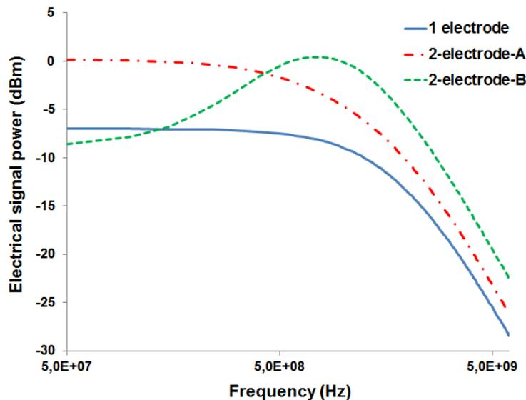
Figure 3- 29: Electrical bandwidth for the three RSOA configurations.
