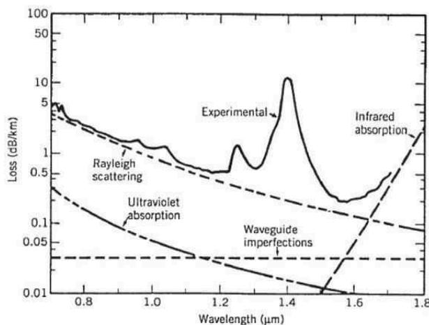
Figure 1- 18 : Loss spectrum of singlemode fiber. The wavelength dependence of several fundamental loss mechanisms is also shown [1].
