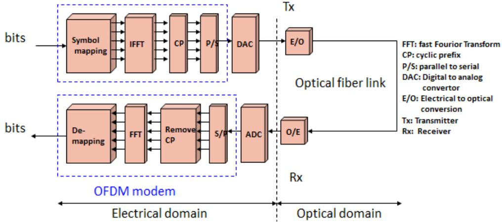
Figure a: Optical OFDM IM-DD transmission system.
