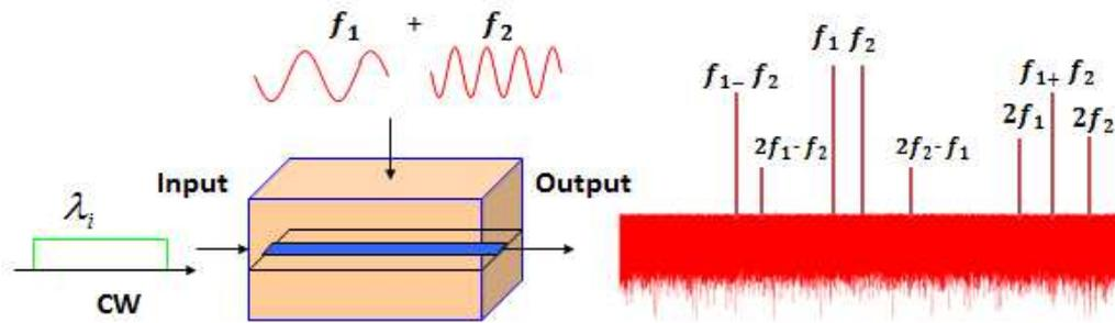
Figure 2- 18 : Principle scheme for RSOA, second order harmonics, 2<sup>nd</sup>, and 3<sup>rd</sup> order intermodulation products by two input electrical signals at frequencies  $f_1$  and  $f_2$ .
