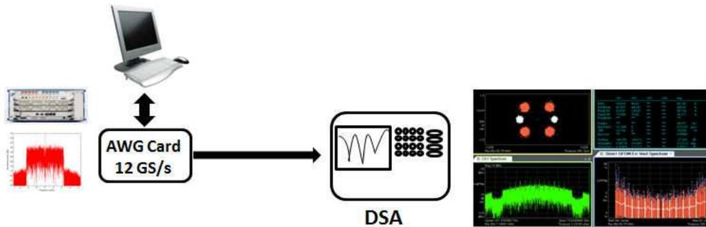
Figure 3- 9 : Experimental setup used for fitting the co-simulation platform in the electrical back to back configuration
