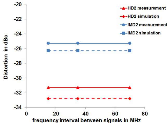
Figure 2- 19 : Simulation and measurement distortion dBc values for 2nd order harmonic and IMD2 signals as function of frequency interval between signals, ( 1 mA input AC current, Input power to the RSOA is 2 dBm, bias current is 60 mA)
