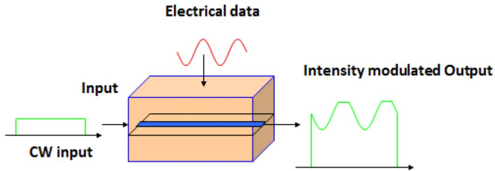
Figure 1- 29: SOA/RSOA intensity modulation principle.
