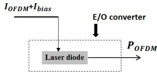
Figure 4- 1 : DFB E/O converter configuration
