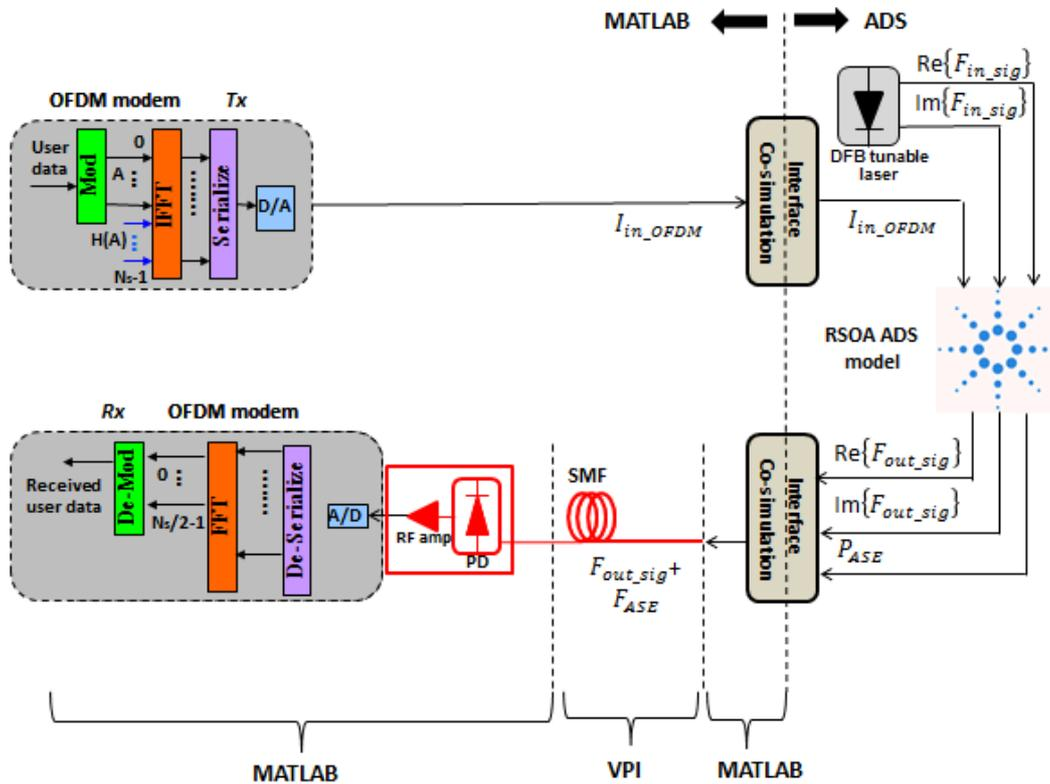
Figure 3- 2 : OFDM IMDD RSOA system co-simulation platform.
