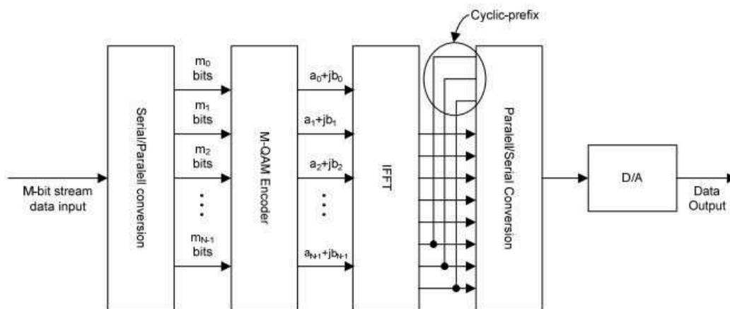
Figure 1- 14 : OFDM transmitter.
