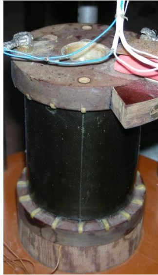
Figure 32 : Superconducting coil used for the application of a magnetic field on the tested composite
