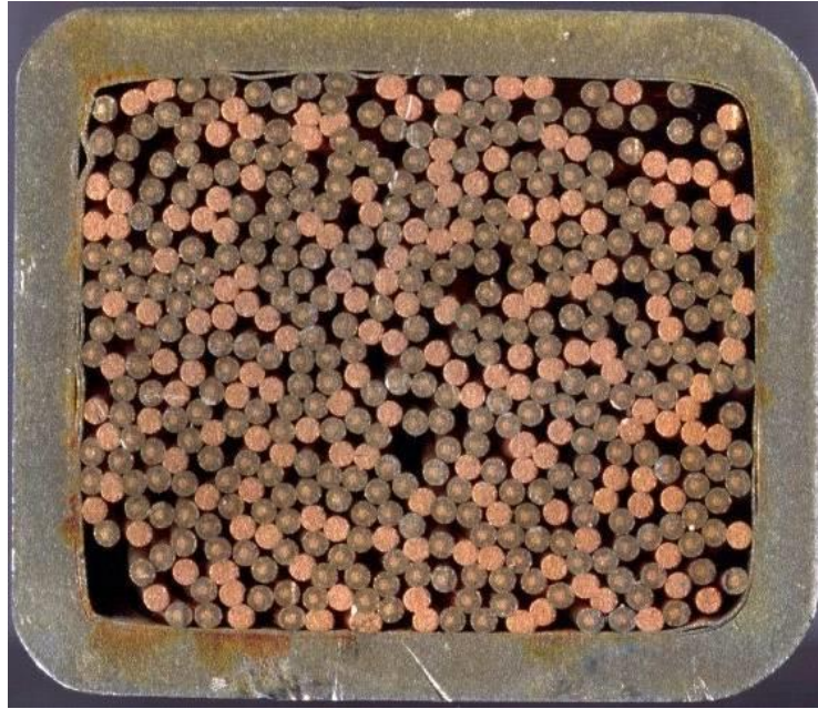
Figure 68 : Photograph of a cross-section of a sample of JT-60SA TF conductor
