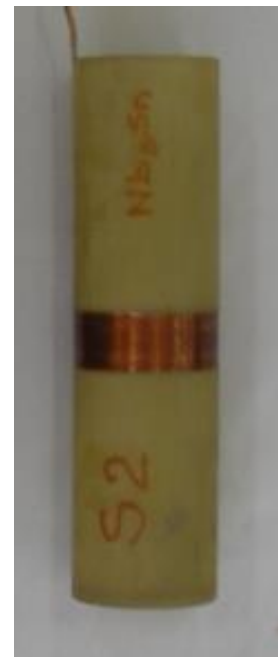
(c) : Example of a sheath holder with the outer pick-up coil wound on it
