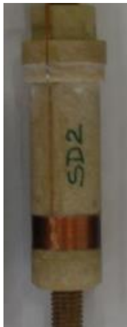
(b) : Example of a finger holder with the inner pick-up coil wound on it
