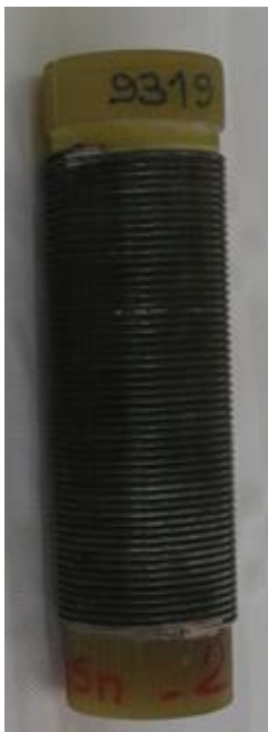
(a) : Example of a sample holder with a composite wound on it
