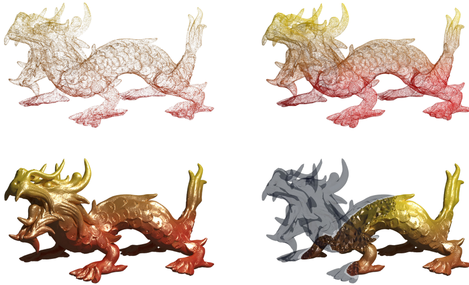
Figure 3.6 – A piecewise linear scalar field constructed on a piecewise linear manifold \mathcal{M} , using linear interpolation. Values are first defined on the vertices of \mathcal{M} (top left), then linearly interpolated at edges (top right), triangles (bottom left), and in tetrahedra (bottom right).
