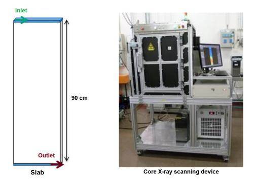
Figure 6.8 – Schematic view of the slab used for the acquisition (left, experimental protocol described in [Lou+18]). It is disposed vertically during the capture. On the right, a typical X-ray scanning device for imaging flow in porous media is shown. Though it was not the case for the captures shown in this chapter, acquisitions can be operated on cores subject to subsurface reservoir conditions, at high pressures (more than 600 bars).
