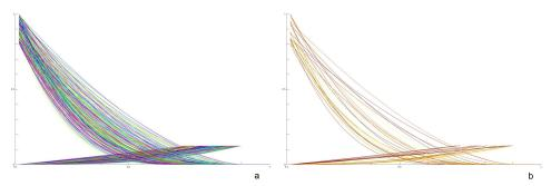
Figure 6.12 – Input relative permeability curves of all 200 simulations (left, with random colors) and for the 25 best selected runs (right, darker is closest to ground truth). No clear pattern was seen that could discriminate relative permeability curves yielding the best fingers.
