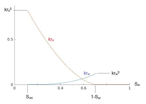
Figure 6.10 – Typical relative permeability curves: for oil (red) and water (blue). In this graph, the abscissa is water saturation  $S_w$ . Intuitively, it represents the extent to which the flow of a phase (say the flow of oil) is inhibited by the presence of another (say the presence of water).
