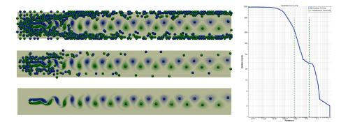
Figure 3.15 – Von Kármán Vortex street phenomenon, showing the turbulence of a fluid flow behind a solid obstacle [Tie16]. Extrema (spheres, blue: minima, green: maxima) of the the orthogonal component of the flow curl are shown (left). The persistence curve (right) shows populations of critical point pairs in the field; by selecting the most persistent ones (those on the right of vertical cuts of the curve), we can define a hierarchy of critical point sets (left, from top to bottom).
