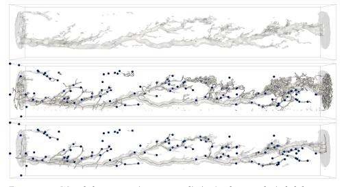
Figure 7.2 – Wormhole structure in porous media (top), whose topological skeleton was extracted by computing the 1-separatrices of the Morse-Smale complex (middle); the most persistent separatrices capture the wormhole structure (bottom). From [PT16].
