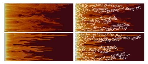
Figure 6.2 – Late time-steps of two Darcy-type simulation runs launched with different model parameters (left column). The ground truth obtained with X-rays is contoured in white (right column, superimposed). Runs exhibit a very chaotic finger geometry.
