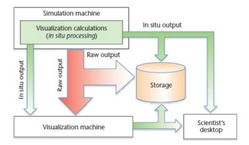
Figure 2.9 – Data flow from simulation to visualization. Two approaches are possible for the analysis of data generated by numerical simulations: post-mortem, whose data flows, displayed in red, are potentially critical analysis bottlenecks if a consequent number of simulation time-steps must be saved; and in-situ (by extension, in-transit), whose data flows, displayed in green, are not an analysis bottleneck. Image from [SA16].
