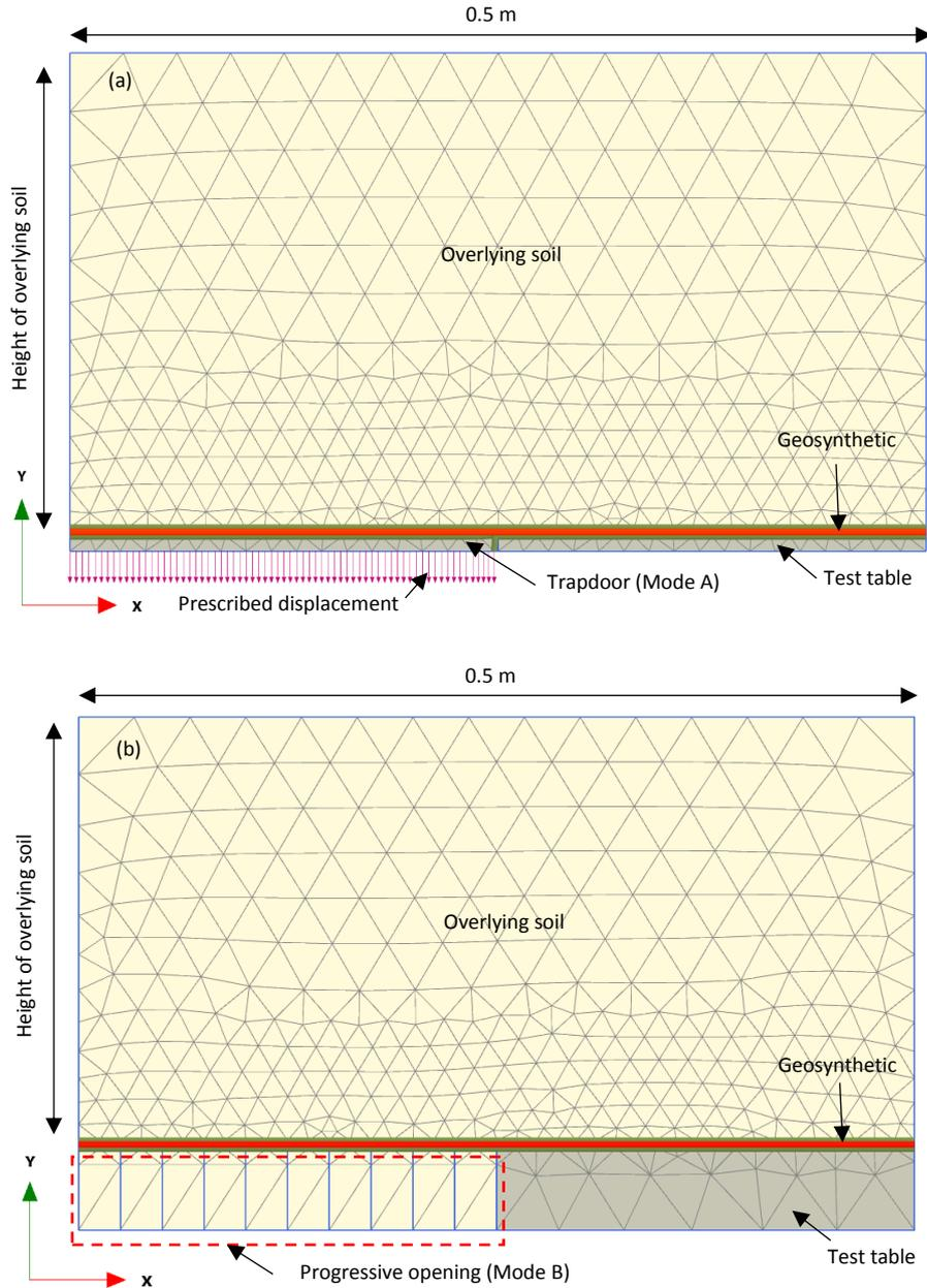
Figure 4.1. Geometrical configuration for the numerical calculation
