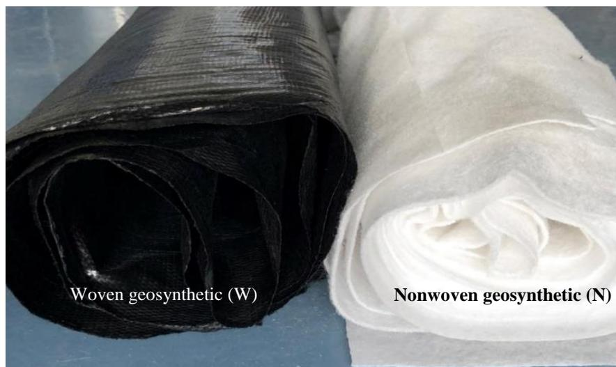
Figure 3.3. Tested geosynthetics
