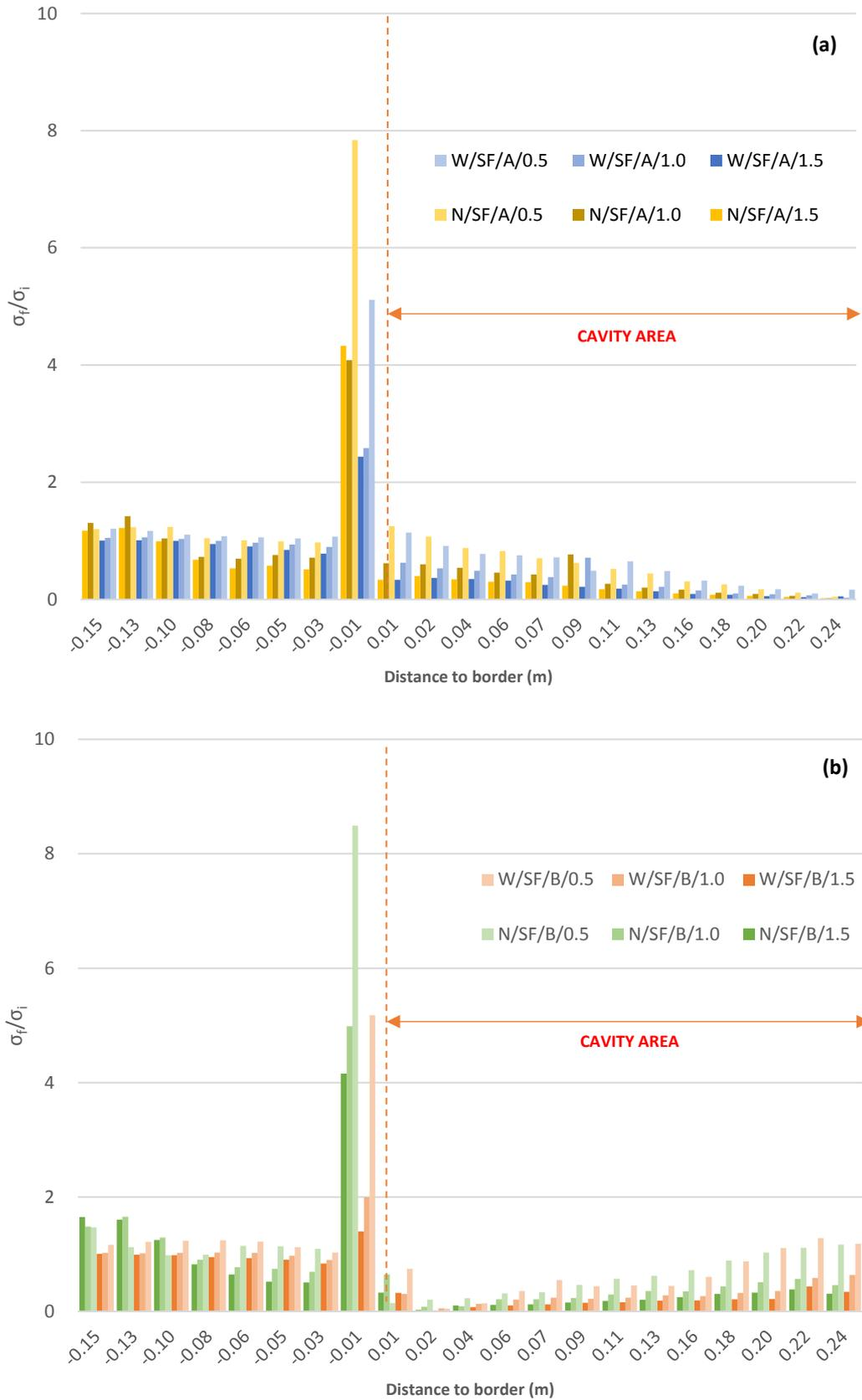
Figure 4.20. Numerical load distribution on cavity calculated for fine sand tests
