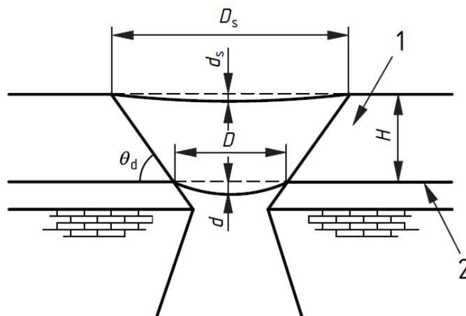
Figure 2.7. Description of parameters for design method (BS8006, 2010)
