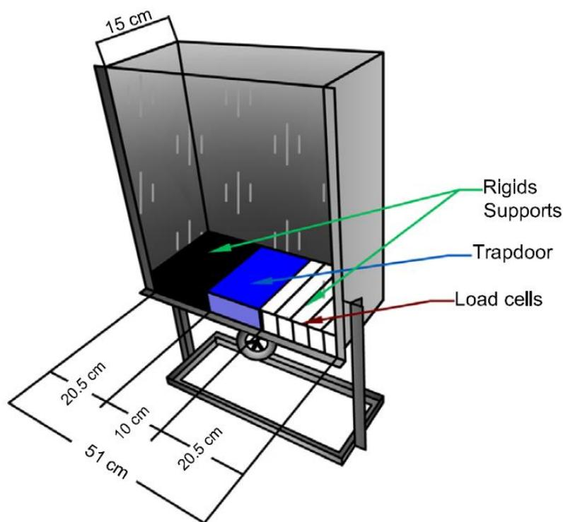
*Figure 2.12. Trapdoor device scheme of Pardo and Sáez (2014)*
