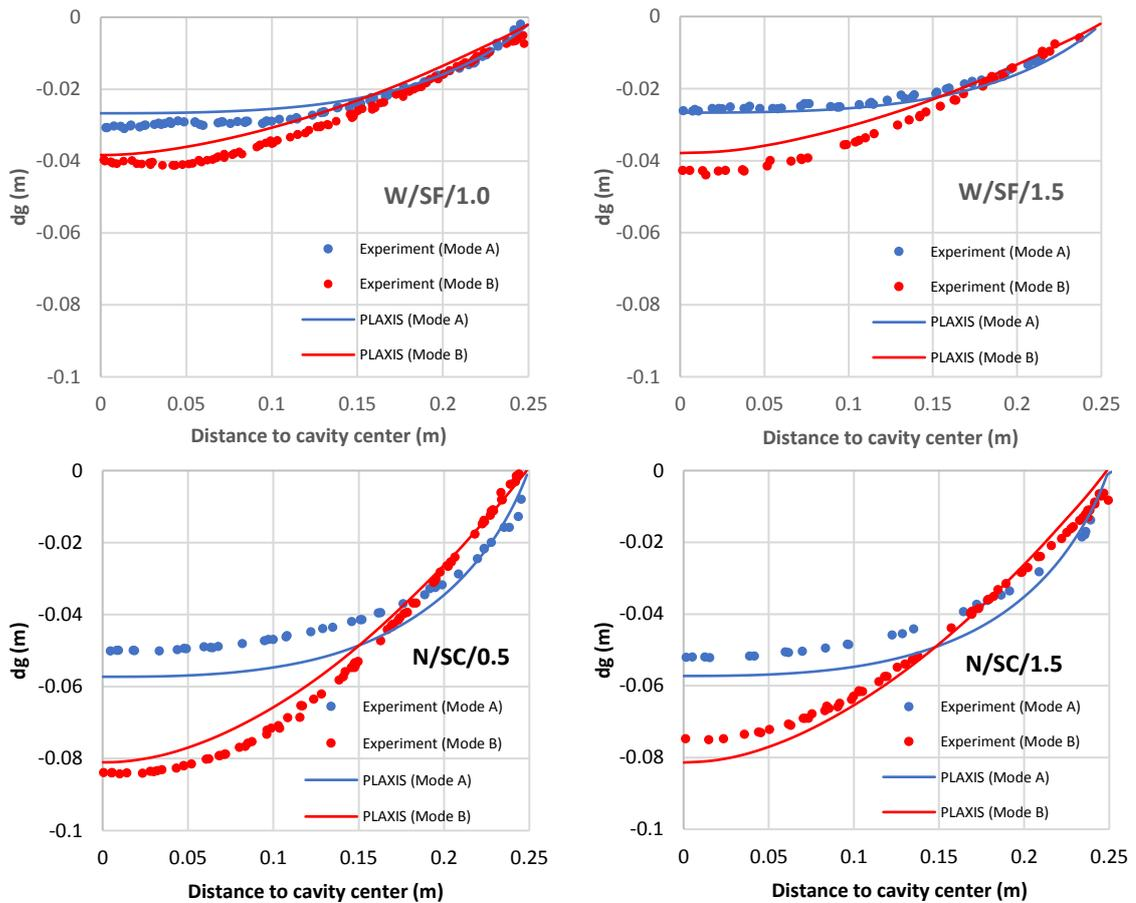
*Figure 4.9. Comparison of deflected geosynthetics between experimental and numerical results*
