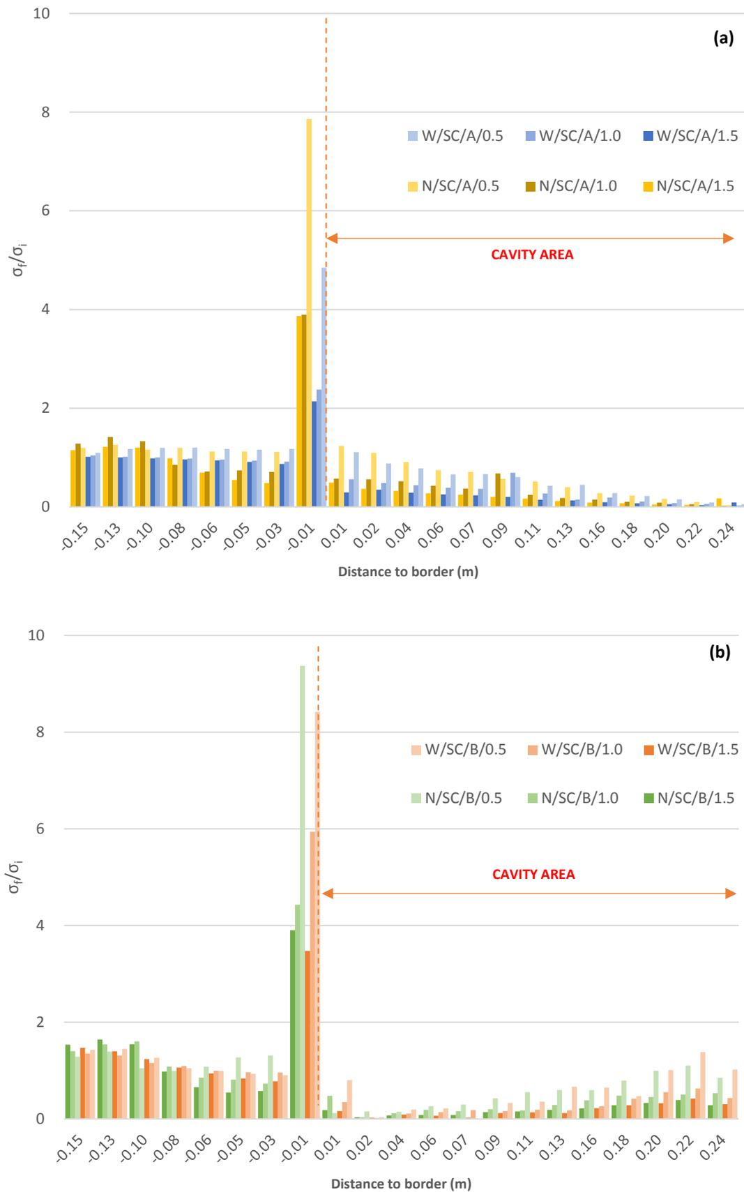
Figure 4.21. Numerical load distribution on cavity calculated for coarse sand tests
