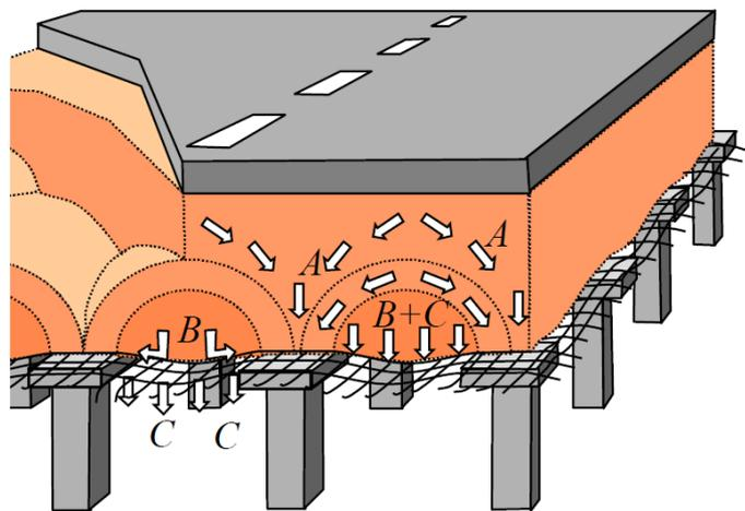
Figure 1.3. Load distribution in piled embankments (Van Eekelen, 2015)
