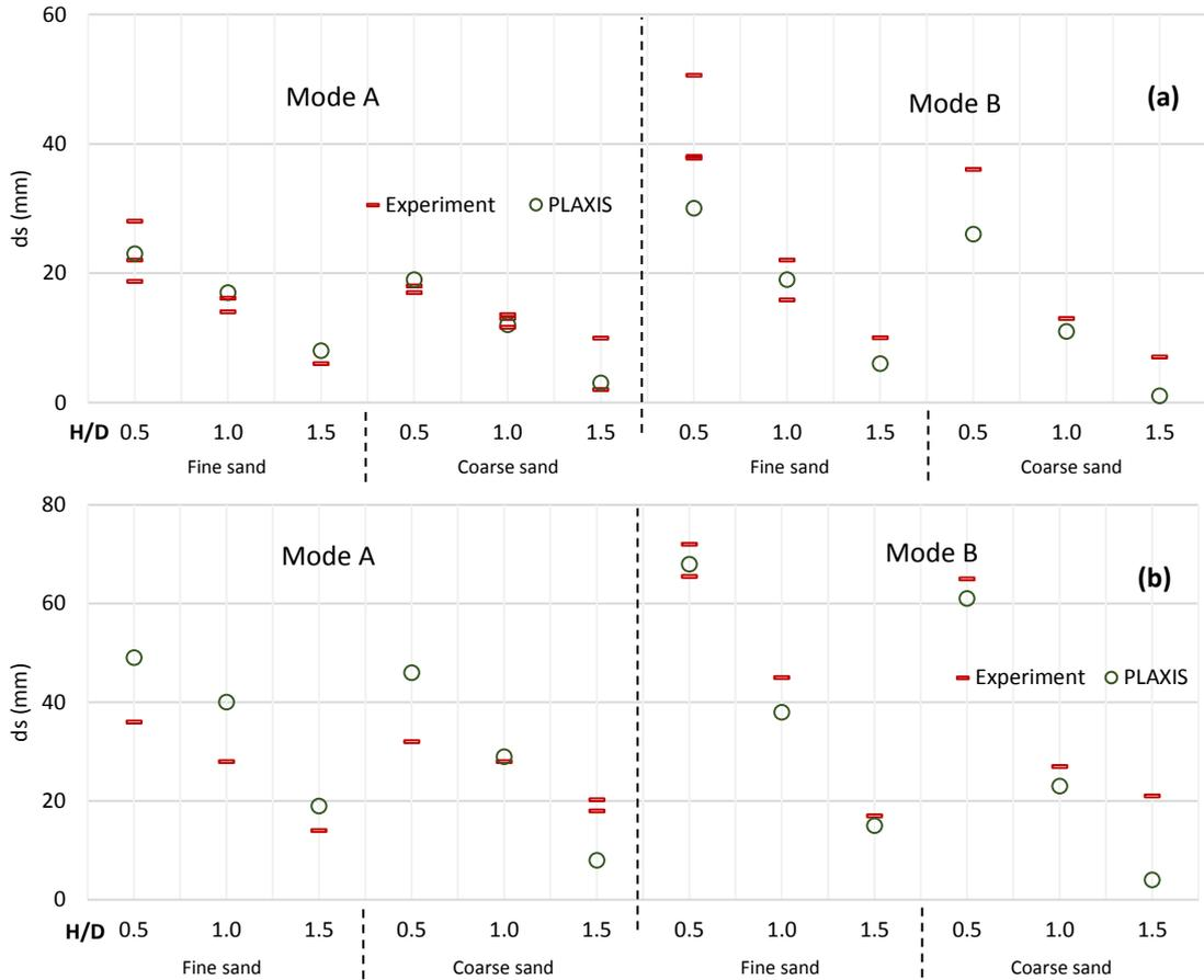
*Figure 4.8. Comparison of surface settlement between experimental and numerical results
