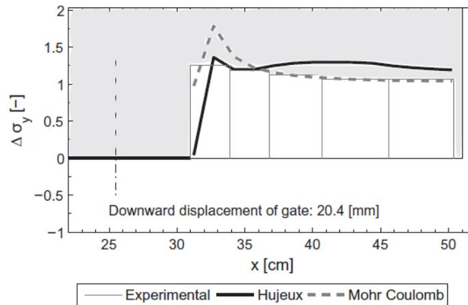
*Figure 2.13. Load distribution on rigid support of the box (Pardo and Sáez, 2014)*
