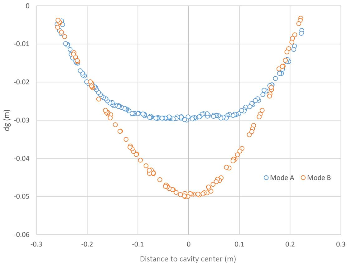
Figure 3.15. A typical comparison of deflected geosynthetic (Fine sand & Woven GSY)
