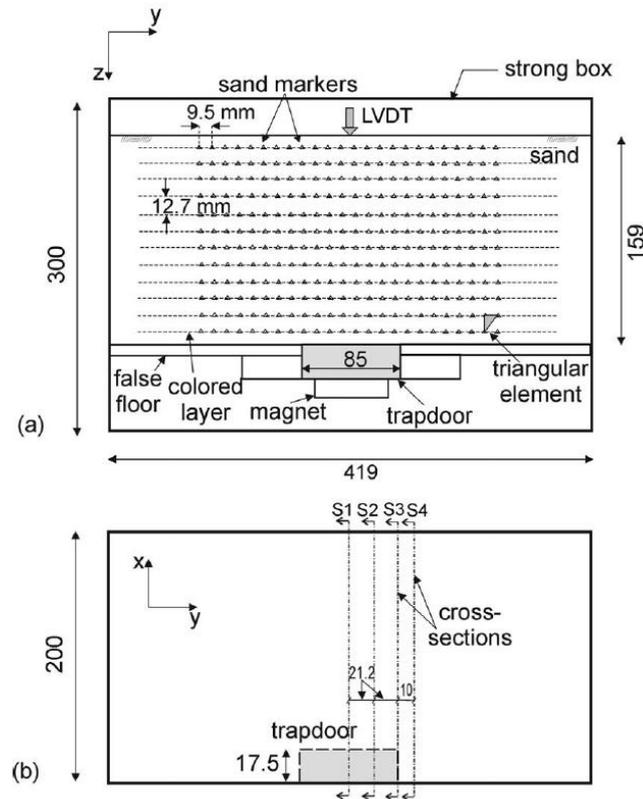
Figure 2.11. Model configuration of Costa et al. (2009)
