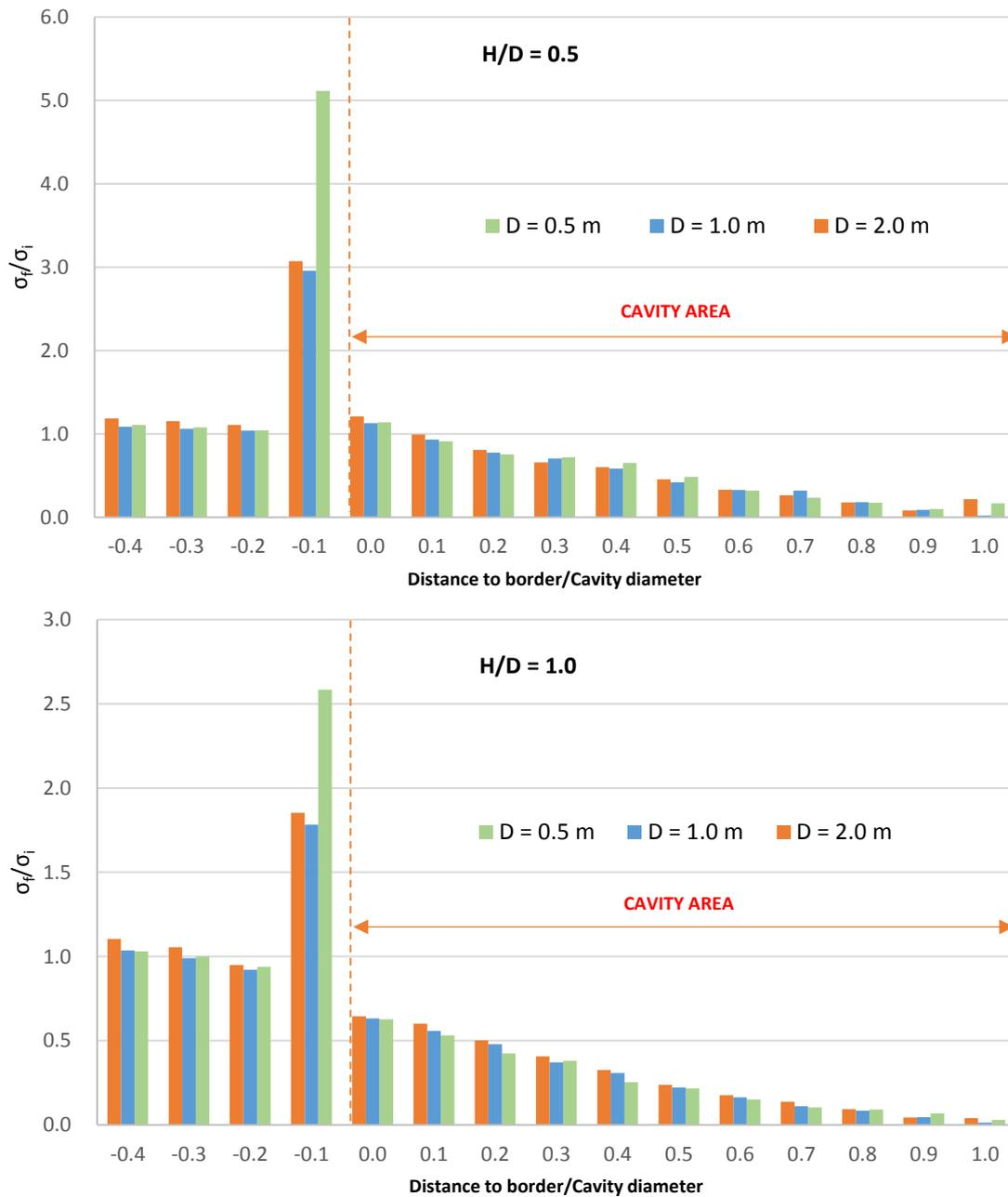
Figure 4.28. Variation of the load distribution due to the cavity diameter variation: Mode A
