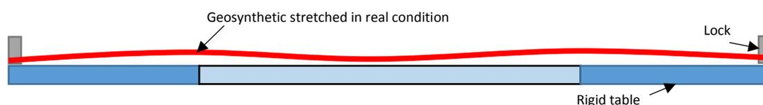
*Figure 3.37. Stretching of geosynthetics on test table*
