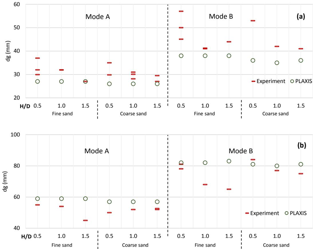
Figure 4.10. Comparison between experimental and numerical results for the maximum geosynthetic deflection
