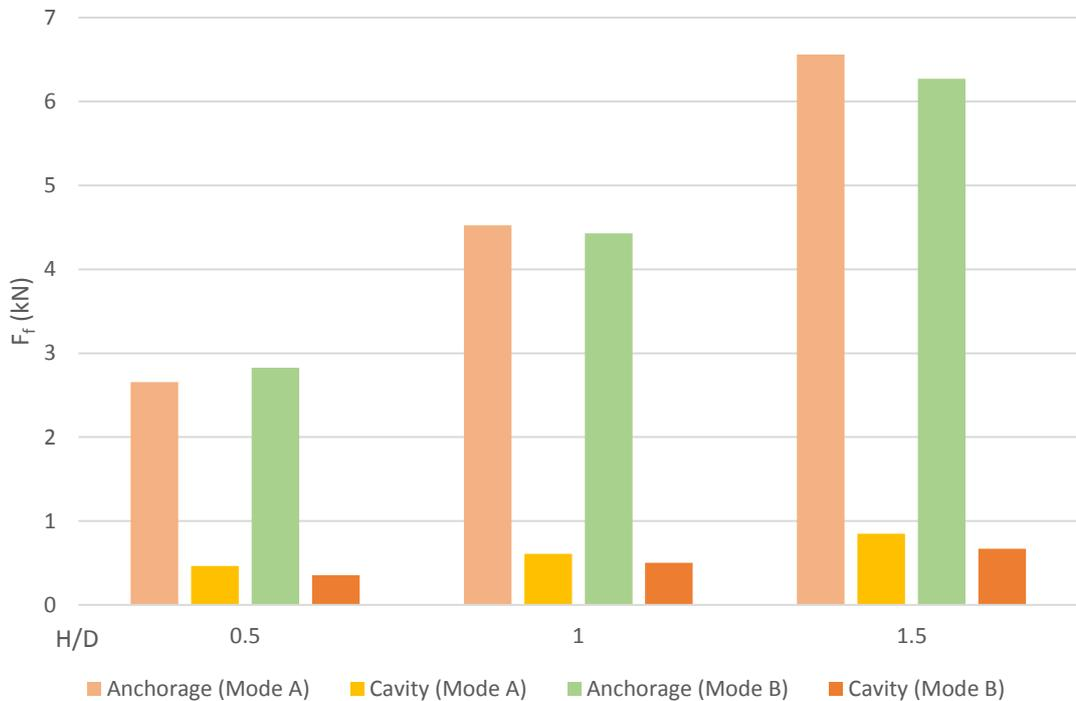
Figure 4.32. Comparison between the final load acting on geosynthetic (Fine sand and Program 2)
