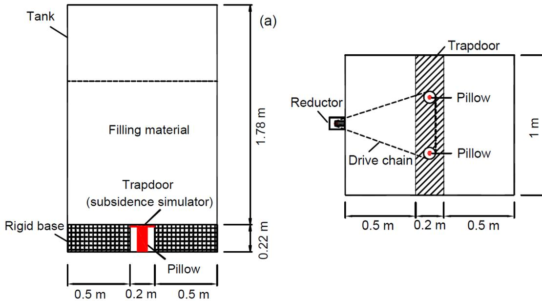
Figure 2.15. Layout of model tests (Zhu et al., 2012)
