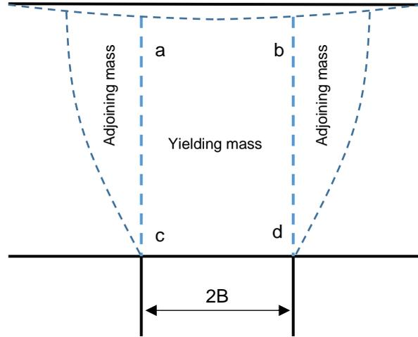
Figure 2.1. The principle of the arching effect (Terzaghi, 1943)
