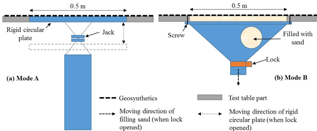
Figure 3.2. Opening methods: trapdoor procedure (a), and progressive procedure (b)
