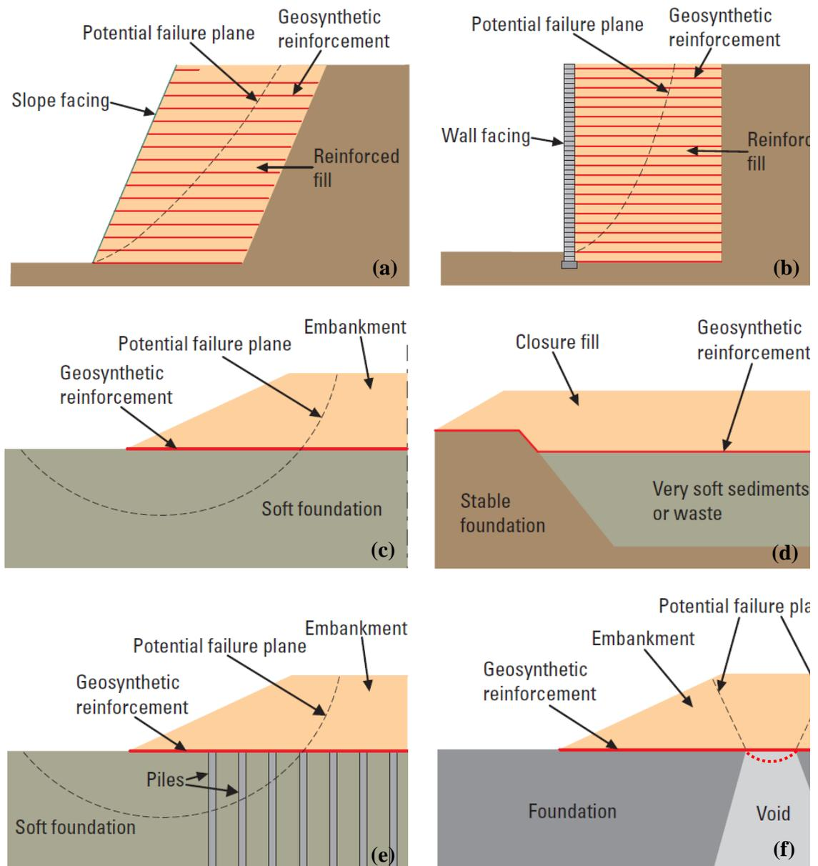
Figure 1.2. Reinforced soil applications
