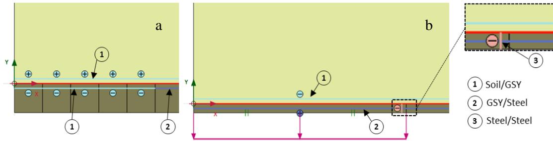
*Figure 4.2. Positions of interface elements used in the numerical modeling
