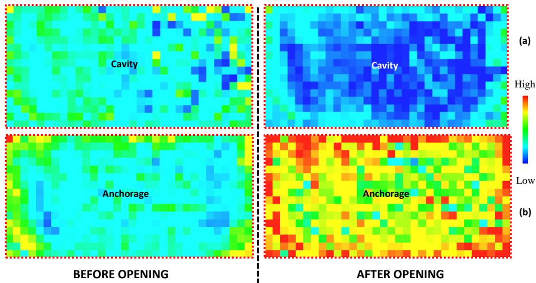
*Figure 3.30. Stress variation measured by TPS comparing to different locations*
