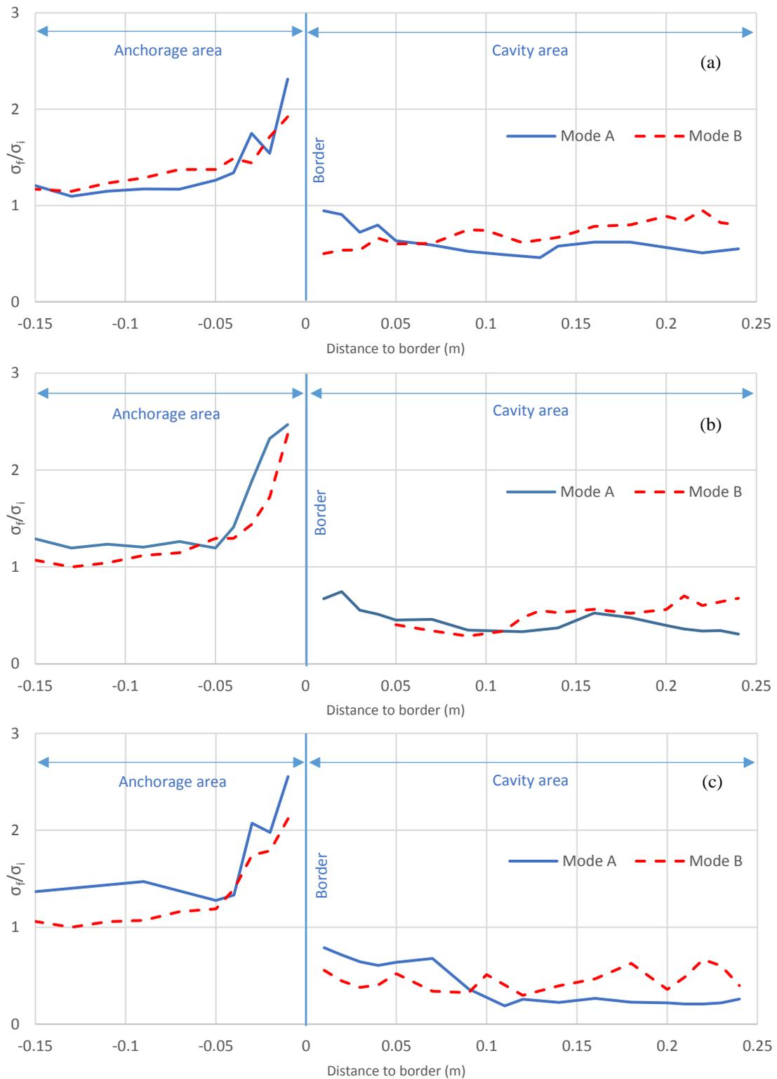
Figure 3.31. Increase of stress after cavity opening (Program 1)
