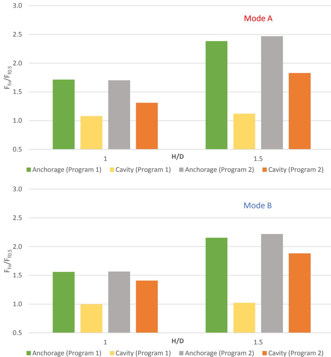
Figure 4.33. Comparison of the load distribution obtained by the numerical models between Program 1 and Program 2
