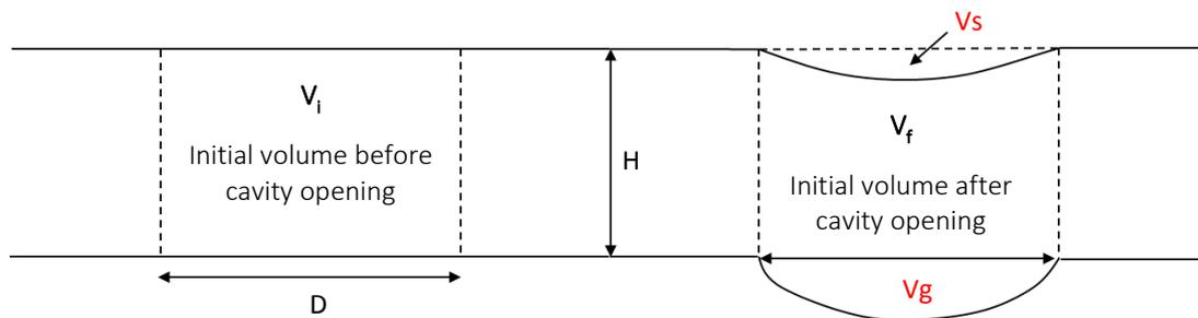
Figure 3.11. Illustration of volumes of soil settlement and geosynthetic deflection
