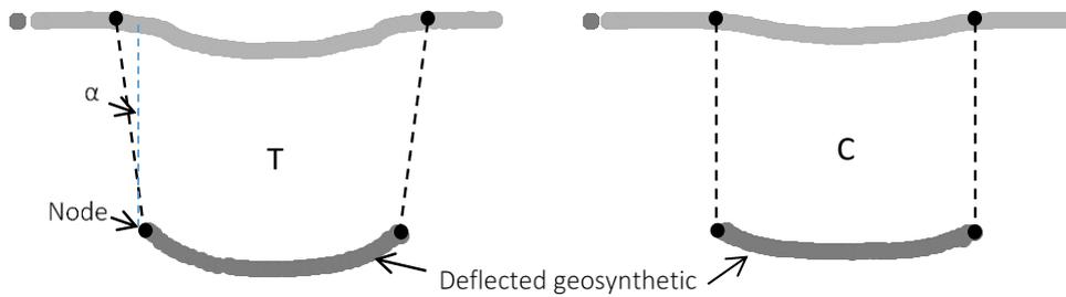
*Figure 3.22. Shape forms of embankment: T – truncated shape, C – cylindrical shape*
