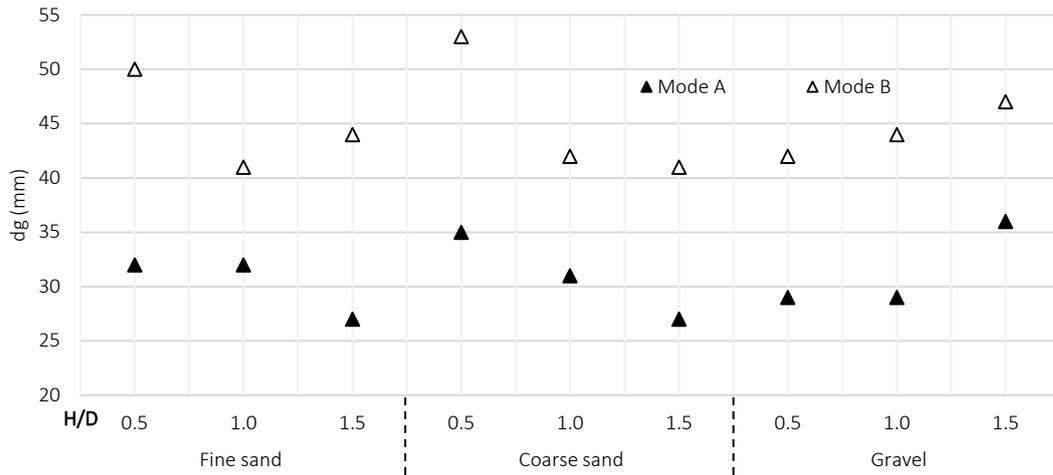
Figure 3.16. Geosynthetic deflection of woven geosynthetic tests
