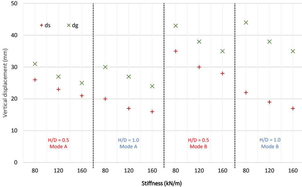
Figure 4.5. Variation of surface settlement and deflected geosynthetics due to changing of geosynthetic stiffness
