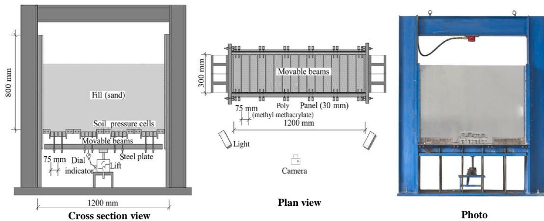
Figure 2.14. Test setup (Rui et al., 2016a)
