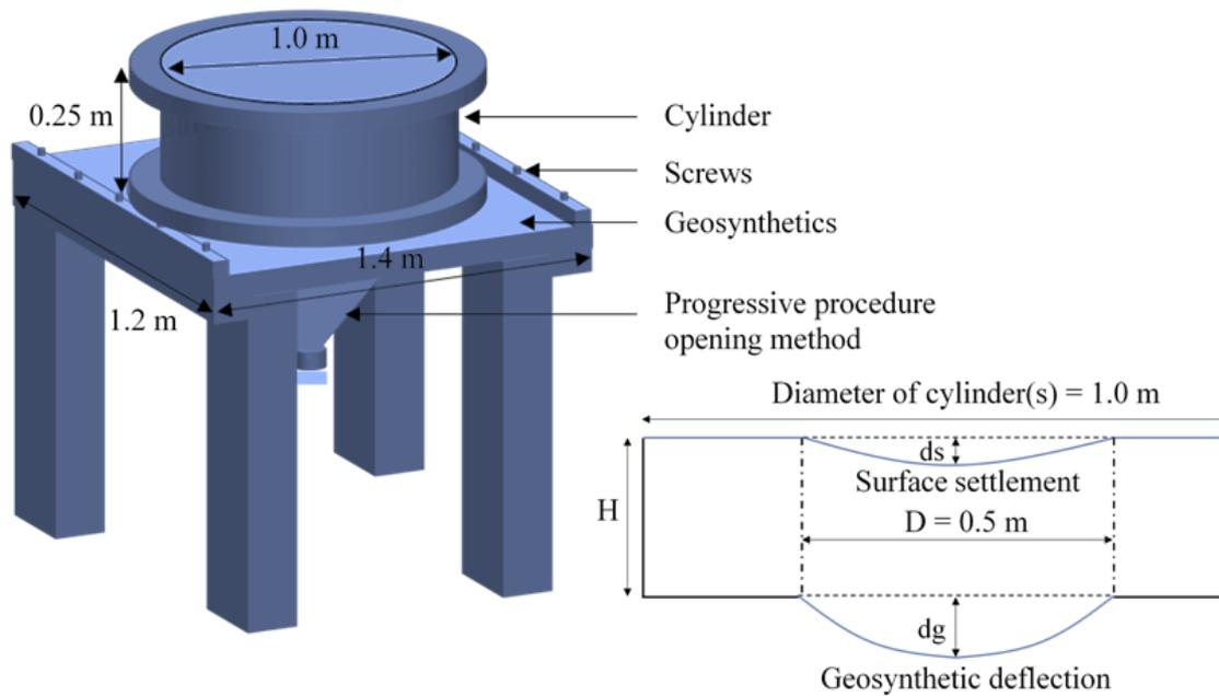
Figure 3.1. Experimental device
