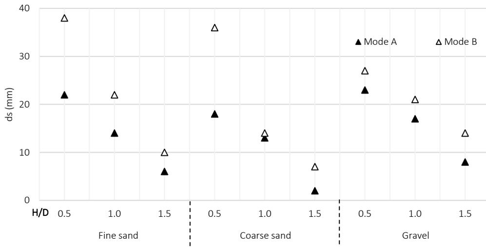
Figure 3.18. Surface settlement of woven geosynthetic tests
