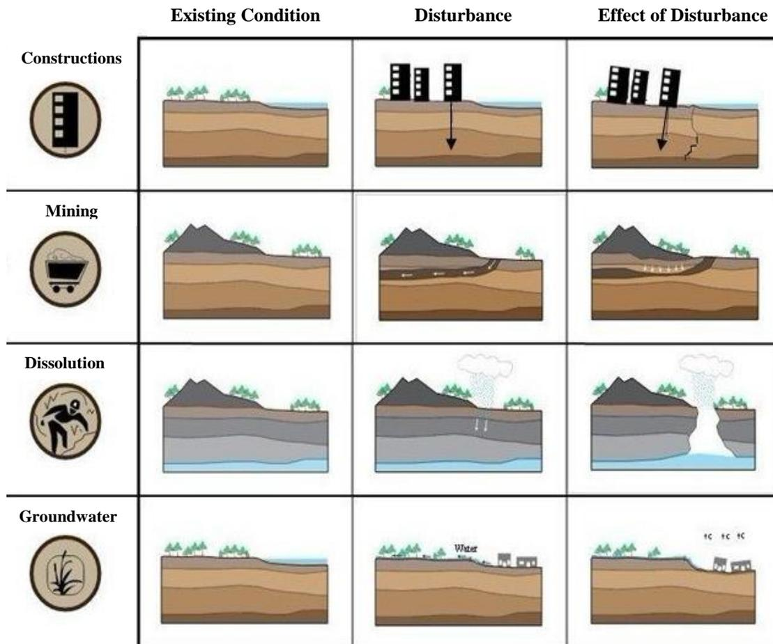
Figure 1.4. Different causes of cavities (URETEK)
