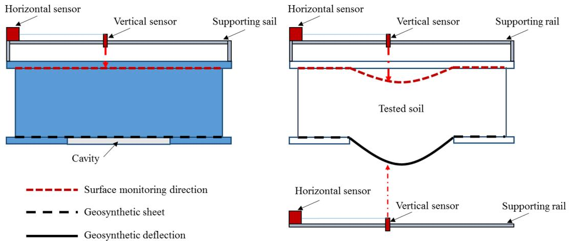
Figure 3.4. Location of displacement monitoring sensors
