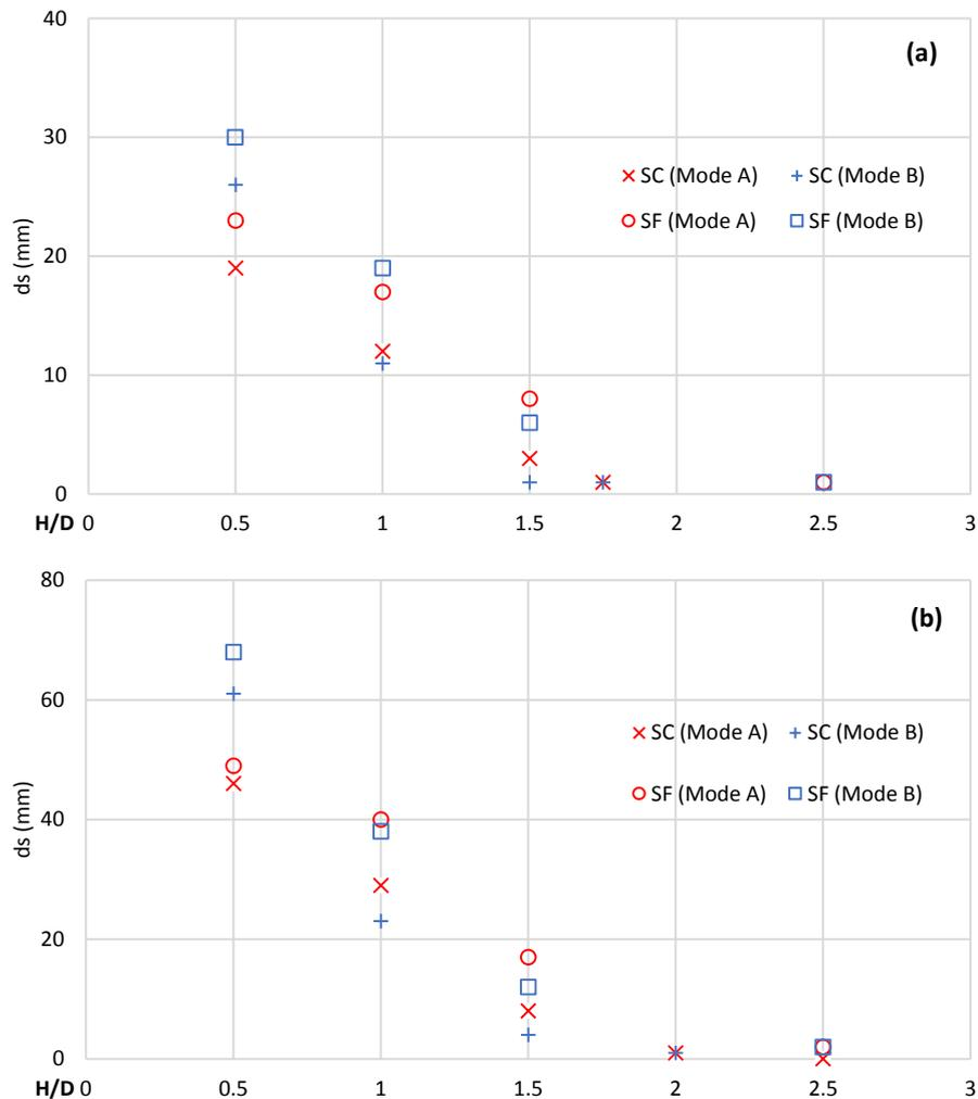
Figure 4.12. Equal settlement plane calculated by PLAXIS
