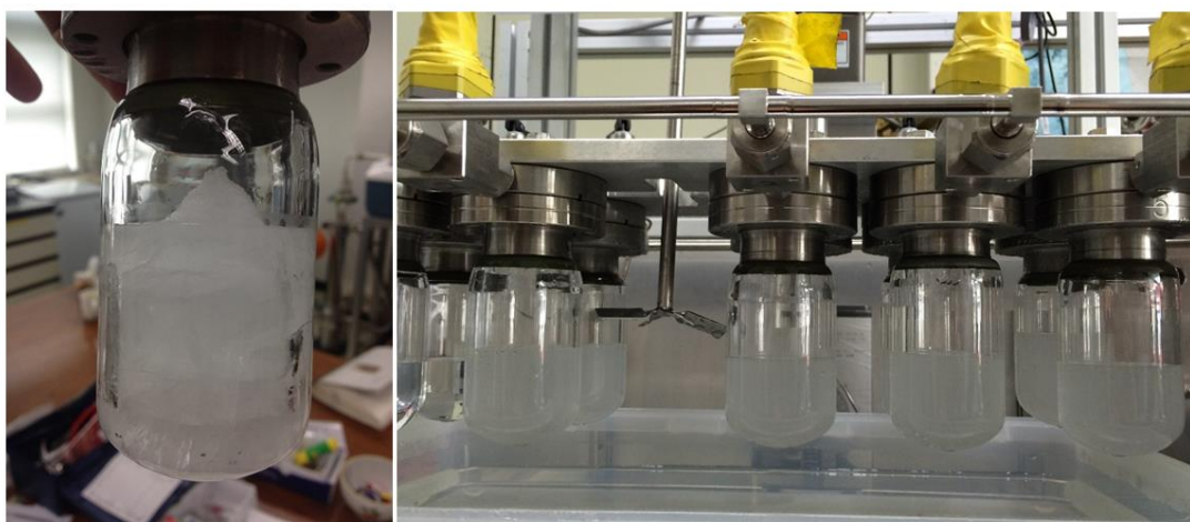
Figure 3.1. Pictures of the melting extraction system for atmospheric \text{CH}_4 concentrations at Seoul National University (SNU) (Photos courtesy of J. Ahn). On the left, the ice sample stored in the chamber before melting. On the right, the multiple chambers containing the melted samples. The principle of wet extraction for \text{CH}_4 is similar to that for \text{CO}_2 .
