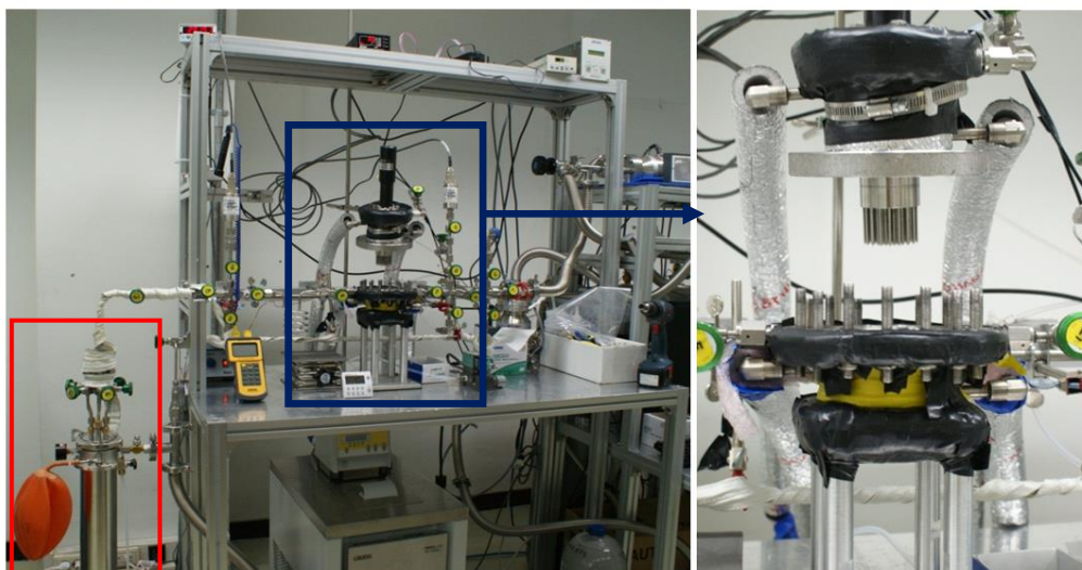
Figure 3.4. The picture on the right shows the dry extraction system line at SNU. The red box indicates the six sample tubes stored in He-closed cycled refrigerator at \sim 10.5 K. The picture on the right show the needle crusher and the chamber where an ice sample is stored.
