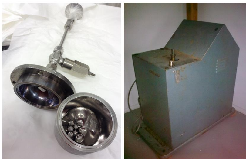
Figure 3.3. The ball mill chamber where an ice sample is crushed containing the eight stainless-steel balls (left) and the vertical crusher (right) located in a walk-in freezer.
