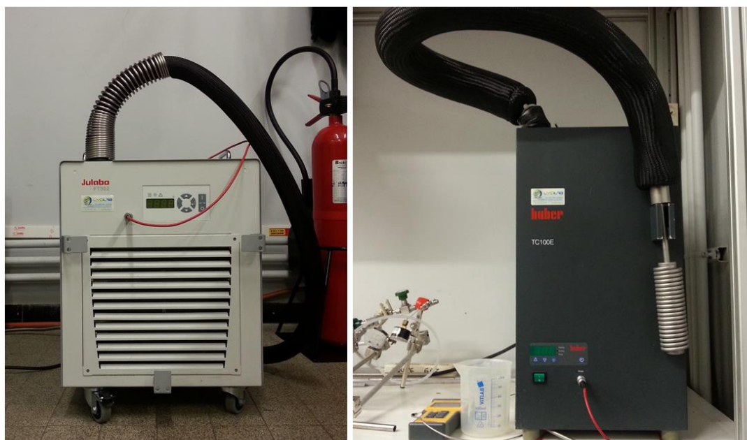
Figure 4.6. Two cooling systems, FT902 Immersion Cooler (left) and Huber TC100E (right)
