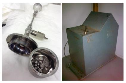
**Figure 3.3.** The ball mill chamber where an ice sample is crushed containing the eight stainless-steel balls (left) and the vertical crusher (right) located in a walk-in freezer.
