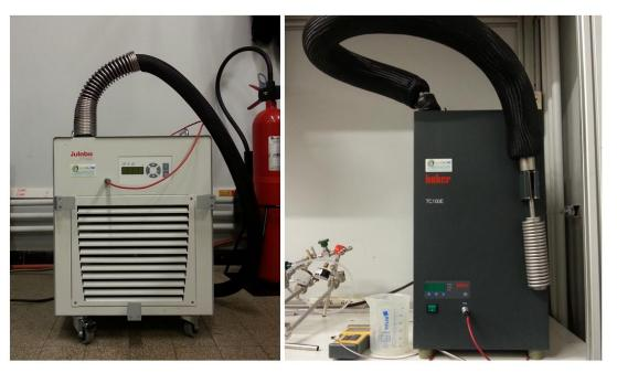
Figure 4.6. Two cooling systems, FT902 Immersion Cooler (left) and Huber TC100E (right)
