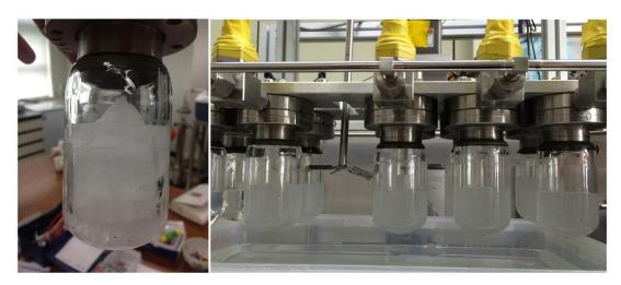
**Figure 3.1.** Pictures of the melting extraction system for atmospheric CH<sub>4</sub> concentrations at Seoul National University (SNU) (Photos courtesy of J. Ahn). On the left, the ice sample stored in the chamber before melting. On the right, the multiple chambers containing the melted samples. The principle of wet extraction for CH<sub>4</sub> is similar to that for CO<sub>2</sub>.
