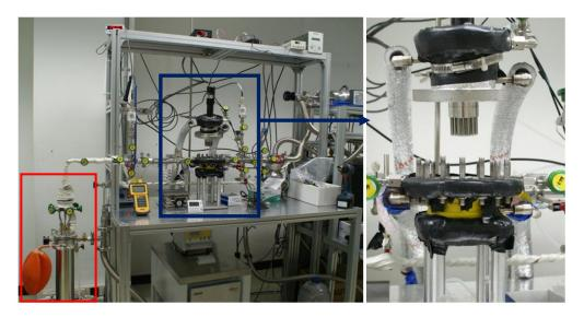
**Figure 3.4.** The picture on the right shows the dry extraction system line at SNU. The red box indicates the six sample tubes stored in He-closed cycled refrigerator at ~10.5 K. The picture on the right show the needle crusher and the chamber where an ice sample is stored.
