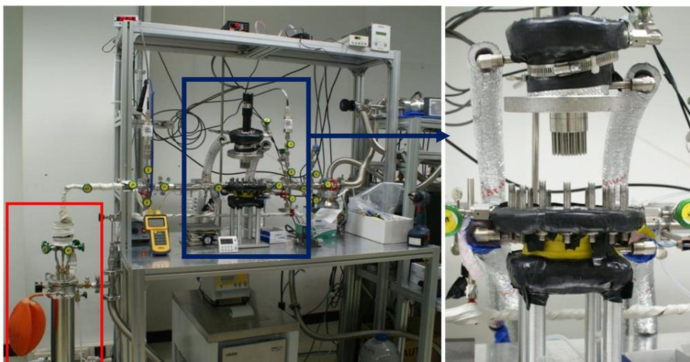
**Figure 3.4.** The picture on the right shows the dry extraction system line at SNU. The red box indicates the six sample tubes stored in He-closed cycled refrigerator at ~10.5 K. The picture on the right show the needle crusher and the chamber where an ice sample is stored.
