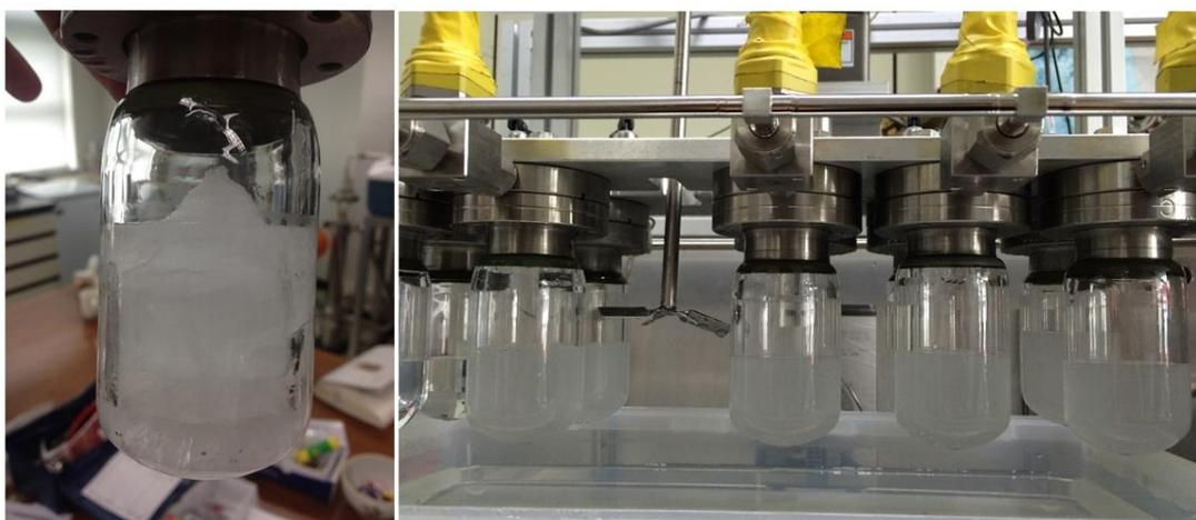
**Figure 3.1.** Pictures of the melting extraction system for atmospheric  $\text{CH}_4$  concentrations at Seoul National University (SNU) (Photos courtesy of J. Ahn). On the left, the ice sample stored in the chamber before melting. On the right, the multiple chambers containing the melted samples. The principle of wet extraction for  $\text{CH}_4$  is similar to that for  $\text{CO}_2$ .
