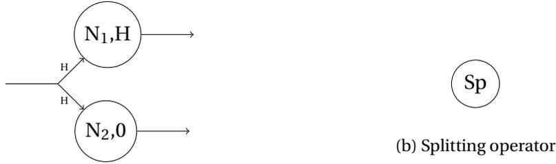
(a) Splitting odd and even spikes from input channel.
