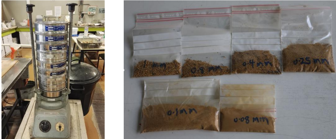
Figure 3.3 Experimental sieves and the retained fractions in wet sieving method
