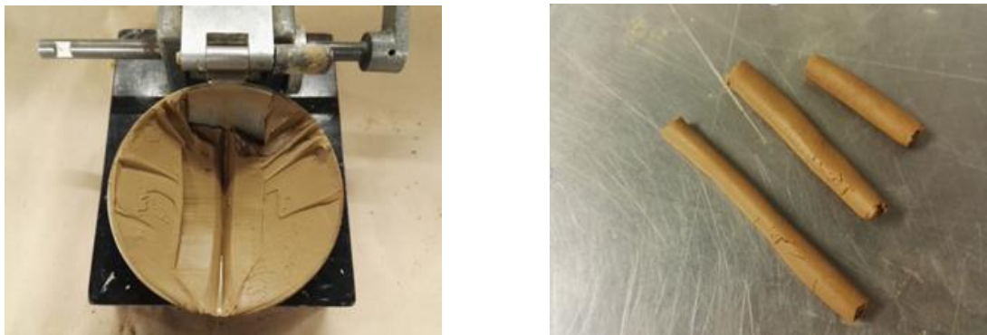
Figure 3.6 Casagrande apparatus and 3 mm diameter rolls without cracking
