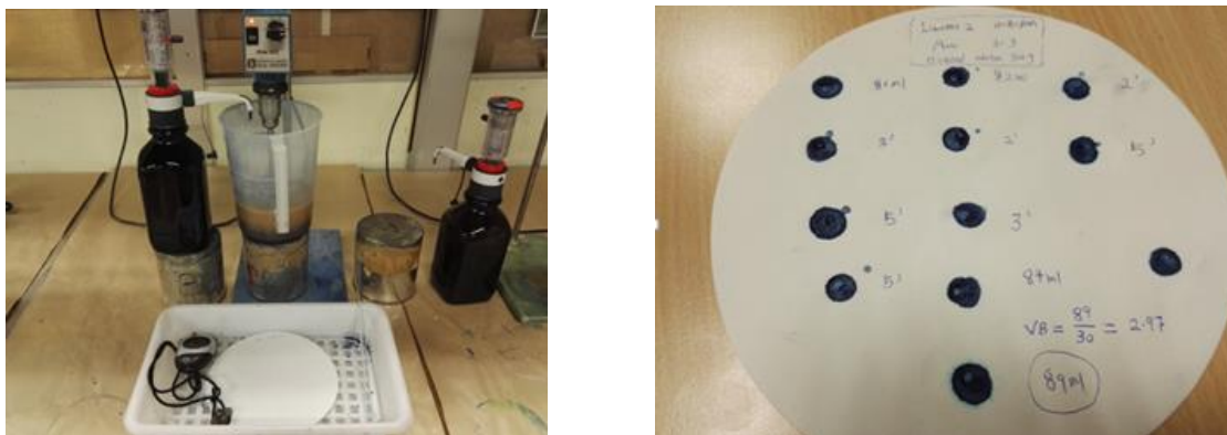
Figure 3.10 Experimental procedure and apparatus for methylene blue value test
