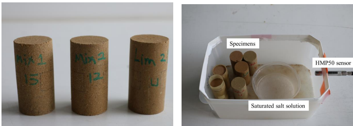
Figure 4.3 Fabricated samples and their conditioning process using saturated salt solutions
