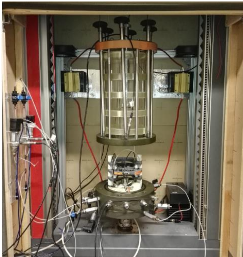
Figure 4.4 Home designed experimental apparatus for loading-unloading triaxial tests
