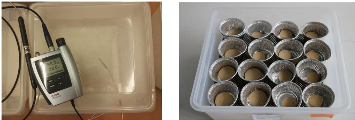
Figure 3.42 Experimental apparatus and samples for isothermal sorption-desorption test using desiccator method
