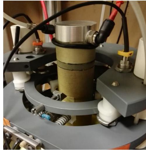
Figure 4.4 Home designed experimental apparatus for loading-unloading triaxial tests
