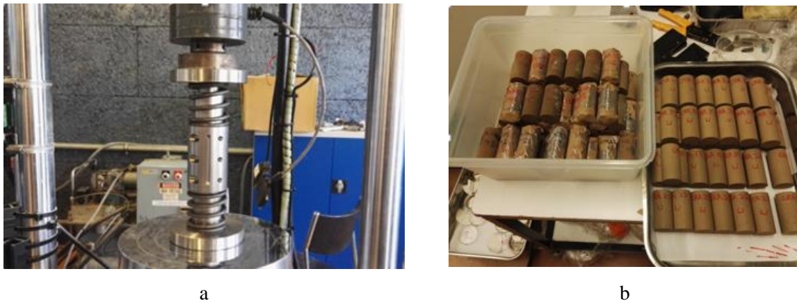
Figure 3.20 (a)Experimental set-up (b) Compacted specimens wrapped with filter paper
