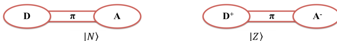
Illustration V 2. Representative illustration of the two basis states of a dipolar dye: the neutral |N\rangle and the zwitterionic |Z\rangle
