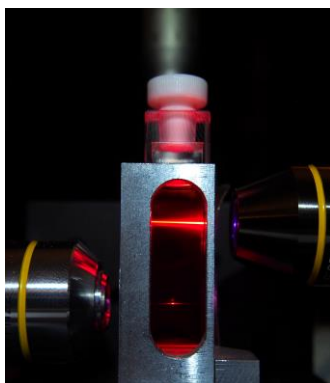
Figure I 3. Difference between the spatial resolution in one-photon (upper part, \lambda_{exc} = 405 \text{ nm} ) and two-photon (lower part, \lambda_{exc} = 1050 \text{ nm} ) process
