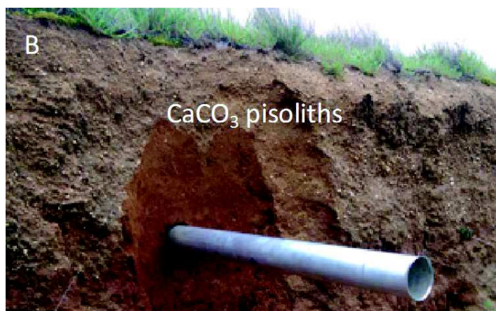
Figure 4-18. Kerarbury Pit, south face, Kerarbury System. A) Upper portion of profile (sampled); B) Surface layer showing sampling location and \text{CaCO}_3 pisoliths embedded in the top 60 cm of the profile
