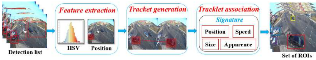
Figure 5.5: Description of tracklet steps. Given a set of samples, a feature extraction block allows to define the characteristics of each sample. The latter is characterized by a position and an appearance information determined by a color histogram (HSV). After that, a tracklet generation block is used to construct initial tracklets by association of samples. The association between the samples is done according to calculate IoU overlap and appearance similarity between samples in successive frames. Next, after initial tracklet constructions, we associate the tracklets having similar signatures. A signature contains the characteristics of appearance, position, speed and size. The output of the association step is a set of ROI associated to target objects.
