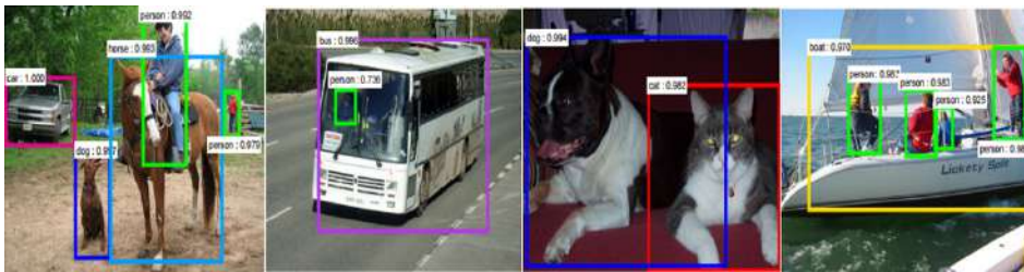
Figure 2.1: Examples of object detection returned by a multi-object detector. Each bounding box color corresponds to a class of objects. Source [Ren 2015c]
