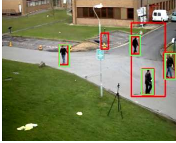
Figure 5.6: The red rectangle presents the area in pixels of the considered RoI, the green rectangle is the area generated by the tracklet tracking algorithm.
