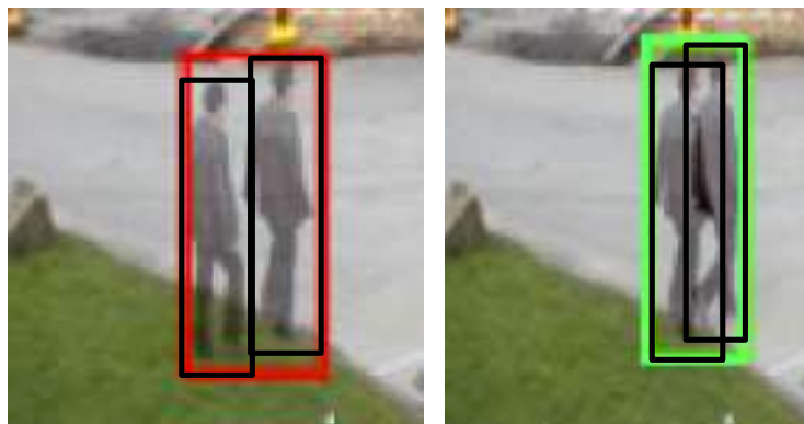
Figure 4.5: Building an annotated interlaced video: Two images extracted from an interlaced video ( D = 2 ) with object bounding boxes in black and interlaced bounding boxes in color.
