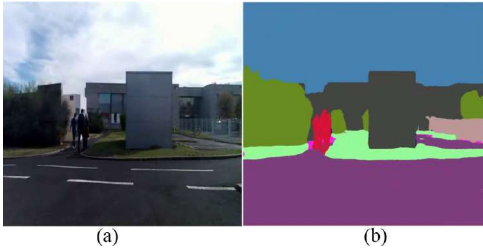
Figure 6.3: Illustration of semantic segmentation task. (a) depicts the input image and (b) is the output one generated by an instance segmentation algorithm.
