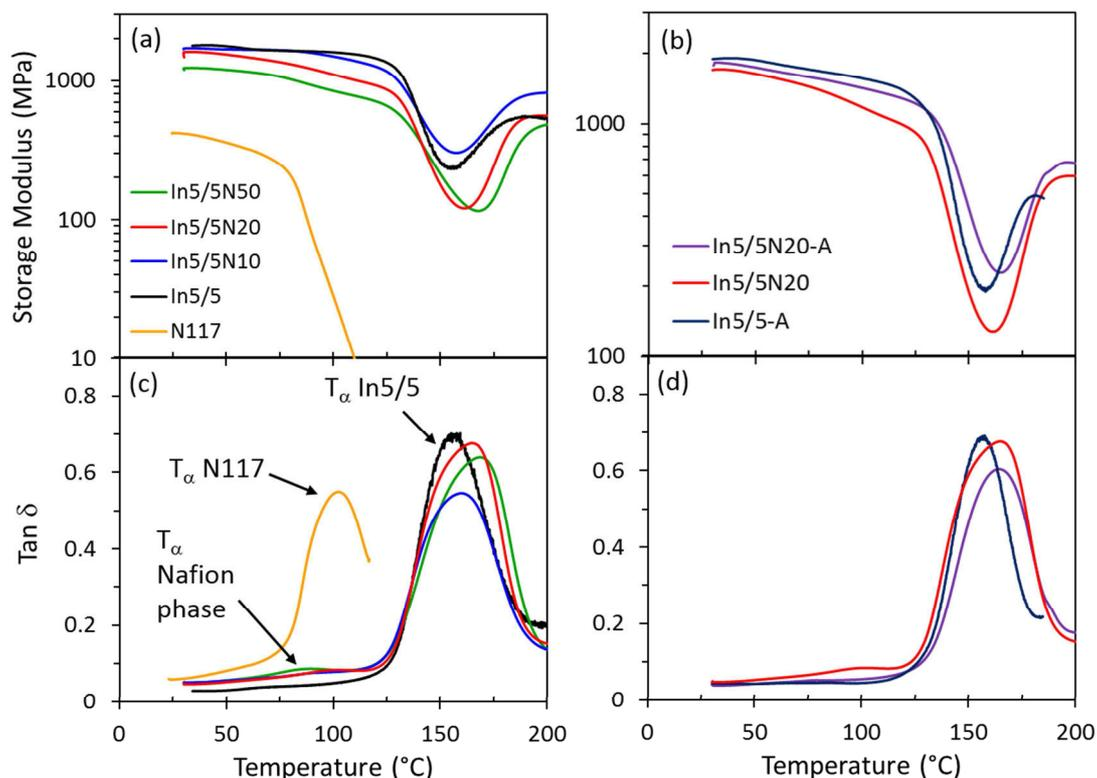
**Figure 2.** (a) Storage modulus and (c)  $\tan \delta$  of blend membranes containing different Nafion content, in comparison with those of Nafion<sup>®</sup> 117 and pristine In5/5 membranes. (b) Storage modulus and (d)  $\tan \delta$  of In5/5N20 and In5/5N20-A membranes. (\* the increase of storage modulus after 160 °C is due to the membrane dehydration and was discussed elsewhere.<sup>14,16</sup>)
