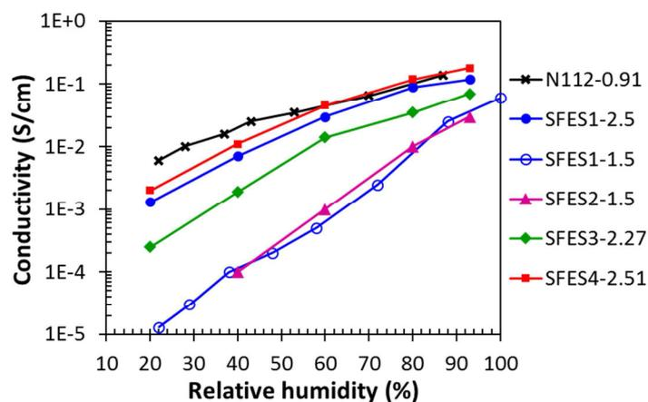
**Figure 3.10.** Proton conductivity vs RH at 80 °C of various random SFES ionomer. The number next to the sample name is IEC.
