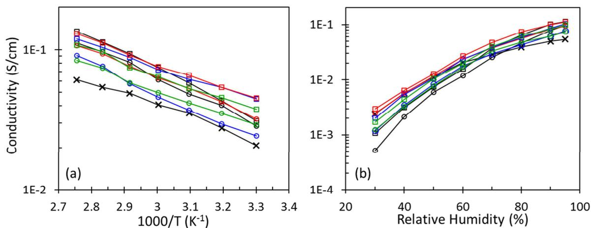
**Figure S3.** Proton conductivity (a) at 95 % RH as a function of 1000/T and (b) at 80 °C as a function of RH of annealed membrane as following: In5/5-A (black ○), In5/5N10-A (blue ○), In5/5N20-A (red ○), In5/5N50-A (green ○), In10/10-A (black □), In10/10N10-A (blue □), In10/10N20-A (red □), In10/10N50-A (green □), in comparison with Nafion 117 (×).
