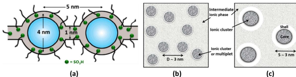
**Figure 2.2.** (a) Cluster-network, (b) inter-particle, and (c) intra-particle core-shell model for morphology of hydrated Nafion. Schemes adapted with permission from ref.<sup>17</sup> Copyright 2004 American Chemical Society.
