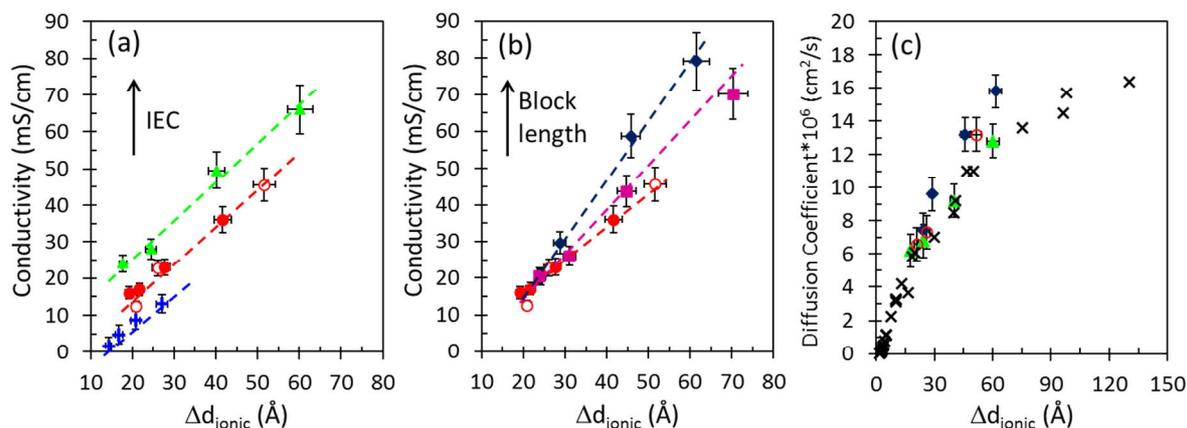
**Figure 8.** Variations of the proton conductivity  $\sigma_i$  (a: IEC-series, b: length-series) and (c) the water self-diffusion coefficient  $D_s$  as a function of the ionic expansion defined by  $\Delta d_{\text{ionic}}$ . Nafion 117 (black  $\times$ ), In2.5/5 (blue  $+$ ), In5/5-1 (red  $\bullet$ ), In5/5-2 (red  $\circ$ ), In7.5/5 (green  $\blacktriangle$ ), In10/10 (purple  $\blacksquare$ ), In15/15 (dark blue  $\blacklozenge$ ).
