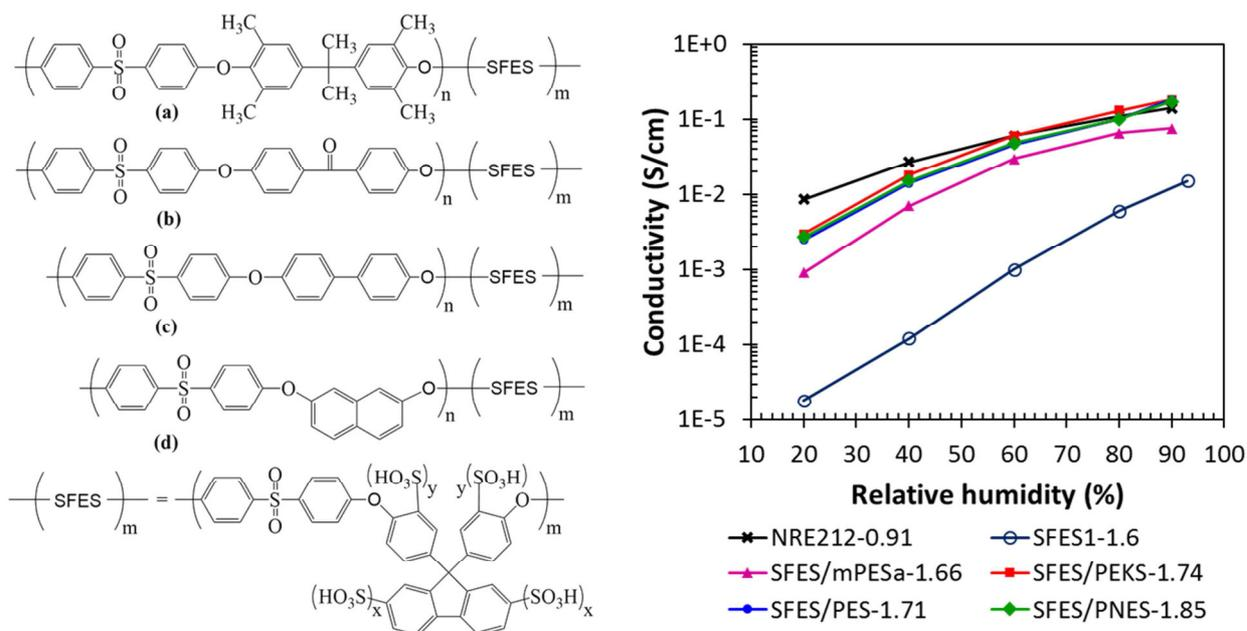
**Figure 3.13.** Chemical structure of SFES-based block copolymers with different hydrophobic blocks (left) and their conductivity measured at 80 °C (right) with similar IEC in comparison to random SFES and Nafion<sup>®</sup> 112 membrane. (a) SFES/mPESa,<sup>96</sup> (b) SFES/PEKS,<sup>95,97,98</sup> (c) SFES/PES,<sup>94</sup> (d) SFES/PNES.<sup>94</sup> The number next to the sample name is IEC.
