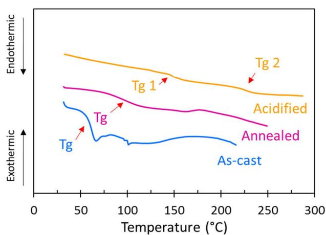
**Figure S1.** DSC diagrams of as-cast, annealed, and acidified In5/5N20 membranes (as cast: membranes membranes in Li form obtained after the casting: it still contains solvent residue therefore the T<sub>g</sub> is so low. Annealed: membranes in Li form resulted after thermal treatment it still contain solvent traces. Acidified: membrane in acidic form obtained after washing with water to completely remove solvent trace and acidification).
