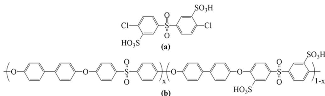
**Figure 3.1.** Chemical structures of (a) SDCDPS and (b) random ionomer as-PES<sub>x</sub>.
