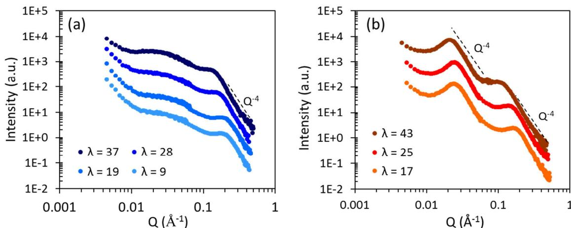
**Figure 3.** Evolution of SANS spectra of the aromatic ionomers upon water content. (a) In5/5-A6 and (b) In5/5-S6. The spectra are shifted vertically for clarity. The dashed lines represent the  $Q^{-4}$  Porod behavior, indicating the presence of a sharp interface at the nanoscale.
