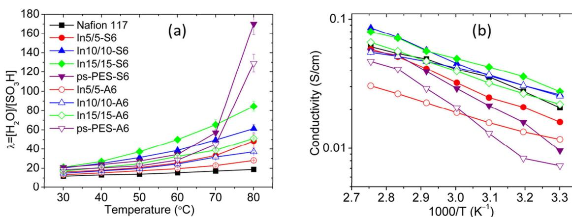
**Figure 7.** (a) Evolution of hydration number ( $\lambda$ ) with the water immersing temperature (b) Evolution of proton conductivity with 1000/T at 95% RH. (Errors limits for conductivities are  $\pm 14\%$ .)
