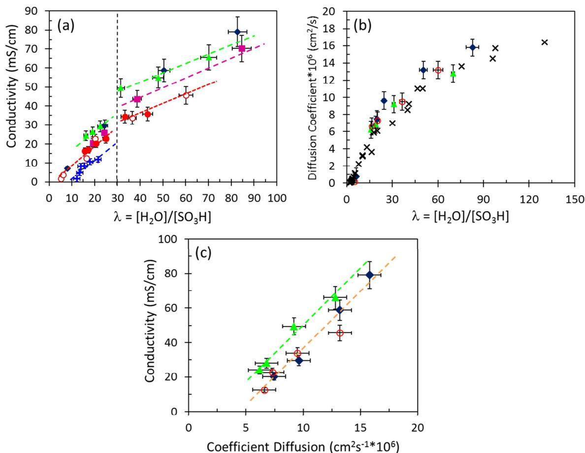
**Figure 7.** (a) Proton conductivity  $\sigma_i$ , (b) water self-diffusion coefficient  $D_s$  vs hydration number, and (c) their correlation. The values of Nafion are also reported for comparison.<sup>47</sup> Nafion 117 (black  $\times$ ), In2.5/5 (blue  $+$ ), In5/5-1 (red  $\bullet$ ), In5/5-2 (red  $\circ$ ), In7.5/5 (green  $\blacktriangle$ ), In10/10 (purple  $\blacksquare$ ), In15/15 (dark blue  $\blacklozenge$ ).
