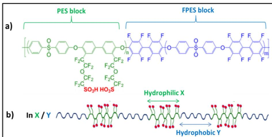
**Figure 1.** a) Chemical formula of ps-PES and FPES blocks. b) Schematic representation of InX/Y ionomers.
