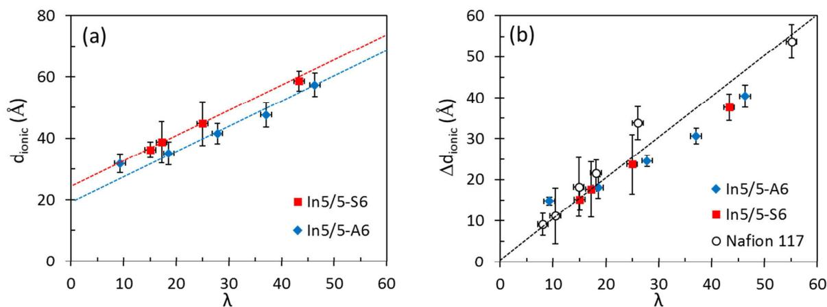
**Figure 4.** (a) Swelling law, i.e., mean separation distances between ionic domains,  $d_{\text{ionic}}$ , as a function of the hydration number  $\lambda$ . (b) Ionic domains mean size,  $\Delta d_{\text{ionic}}$ , as a function of the hydration number. The  $d_0$  values are extrapolated from the swelling law at  $\lambda = 0$ .
