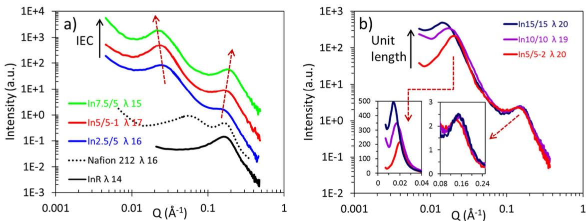
**Figure 2.** SANS spectra of hydrated aromatic block ionomers. (a) IEC-series and (b) Length-series. The spectra are shifted vertically for clarity, and compared to that of random ionomer (InR) and Nafion<sup>®</sup> 212 at similar  $\lambda$ . The SANS profile of Nafion<sup>®</sup> 212 membrane was taken from ref.<sup>39</sup>
