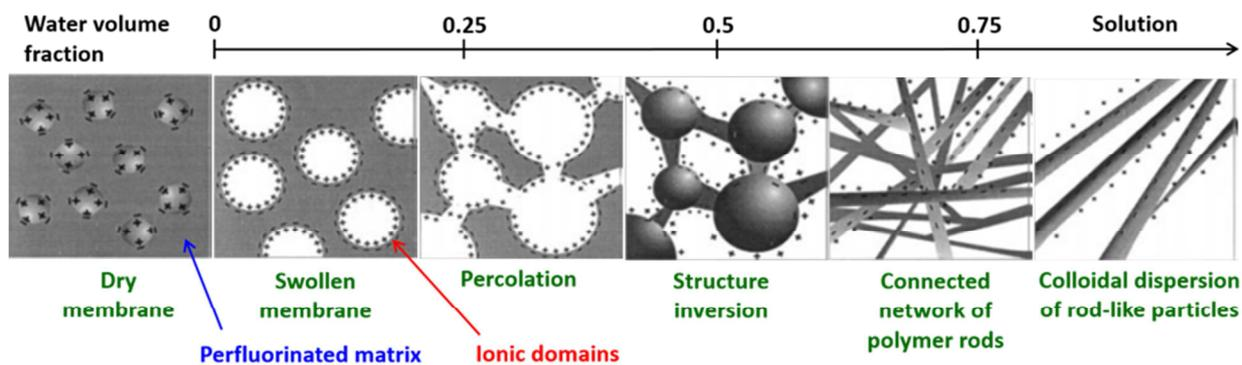
**Figure 2.4.** Schematic representation of the structural evolution as a function of water content. Schemes reprinted and adapted with permission from ref.<sup>46</sup> Copyright 2000 Elsevier.
