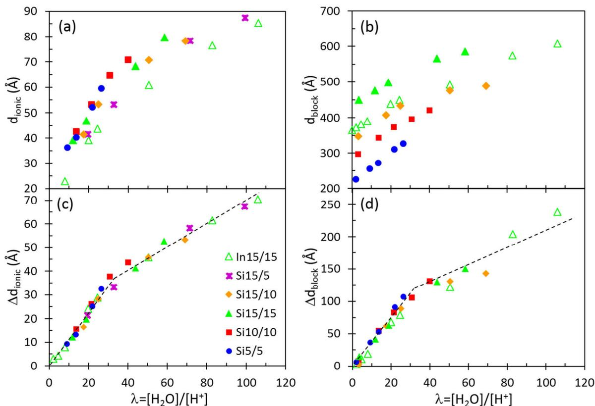
**Figure 7.** Variations of mean separation distances of (a) ionic domains ( $d_{\text{ionic}}$ ), (b) block structures ( $d_{\text{block}}$ ) as a function of  $\lambda$  and their expansions: (c)  $\Delta d_{\text{ionic}}$  and (d)  $\Delta d_{\text{block}}$ .
