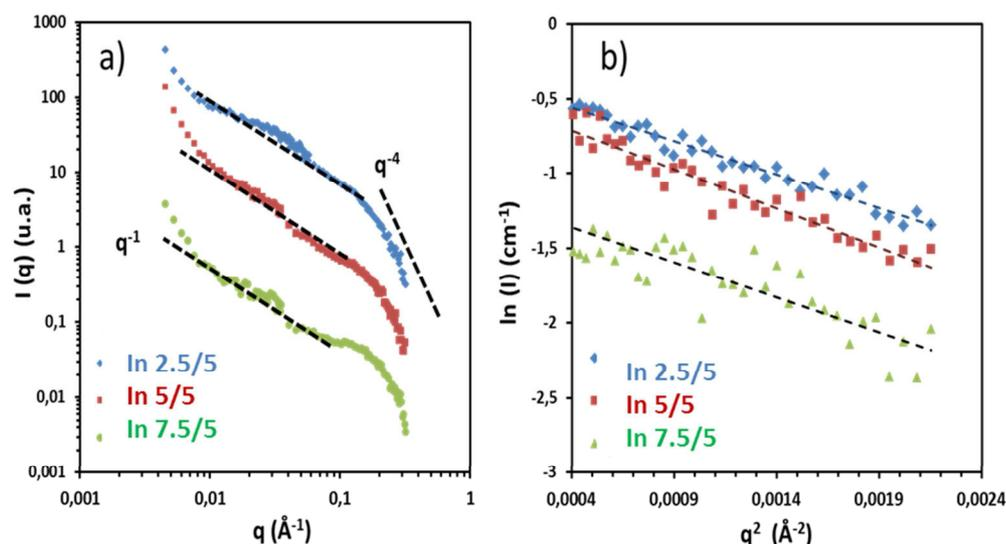
**Figure S6.** a) SANS intensities  $I(q)$  of ionomer solutions in DMSO (1,6 % w/w) as a function of the scattering vector  $Q$ . The  $I(Q)$  curves were shifted for clarity. b) Guinier representation ( $\ln(I)$  vs  $Q^2$ ).
