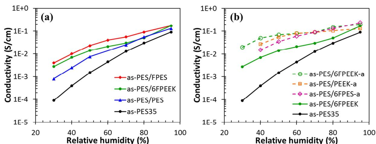
**Figure 3.4.** Proton conductivity vs reduced humidity at 80 °C of (a) not annealed and (b) annealed (marked with suffix -a) SDCDPS-based ionomer membranes. 1) as-PES35,<sup>72</sup> 2) as-PES/PES 10/10 with HFB linked group,<sup>68,73</sup> 3) as-PES/FPES 15/15,<sup>72,74</sup> 4) as-PES/6FPES 15/15,<sup>69</sup> 5) as-PES/PEEK 17/17,<sup>71</sup> 6) as-PES/6FPPEEK 14/14.<sup>70</sup>
