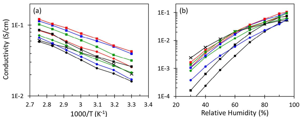
**Figure S2.** Proton conductivity (a) at 95 % RH as a function of 1000/T and (b) at 80 °C as a function of relative humidity of cast membrane as following: In5/5 (black ●), In5/5N10 (blue ●), In5/5N20 (red ●), In5/5N50 (green ●), In10/10 (black ■), In10/10N10 (blue ■), In10/10N20 (red ■), In10/10N50 (green ■), in comparison with Nafion 117 (×).
