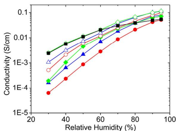
**Figure 11.** Proton conductivity at 80 °C of Nafion 117 (black ■), In5/5-S6 (red ●), In10/10-S6 (blue ▲), In15/15-S6 (green ◆), In5/5-S15 (red ○), In10/10-S15 (blue △), In15/15-S15 (green ◇). (Errors limits for conductivities are  $\pm 14\%$ ).
