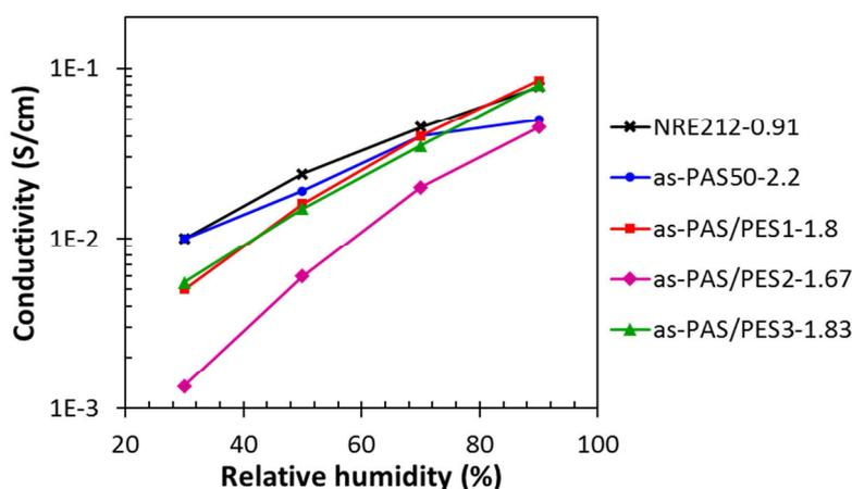
**Figure 3.7.** Conductivity vs RH at 80 °C of random and block copolymers proposed by Jannasch et al.<sup>85-87</sup> The number next to the sample name is IEC.
