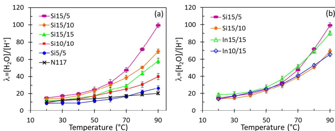
**Figure 8.** a) Water uptake of SiX/Y ionomers in comparison with Nafion<sup>®</sup> 117, and b) Water uptake of SiX/Y ionomers in comparison with InX/Y.
