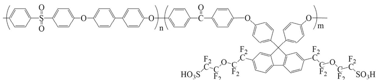
**Figure 3.22.** Chemical structure of multi-block copolymer ps-PEK/PES.
