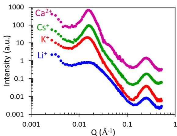
**Figure P1.** SANS profiles of acidified-annealed DMAc-cast In10/10 membranes cast from ionomers in different salt forms. There is a clear impact of the cation on the block superstructure organization (low Q peak).
