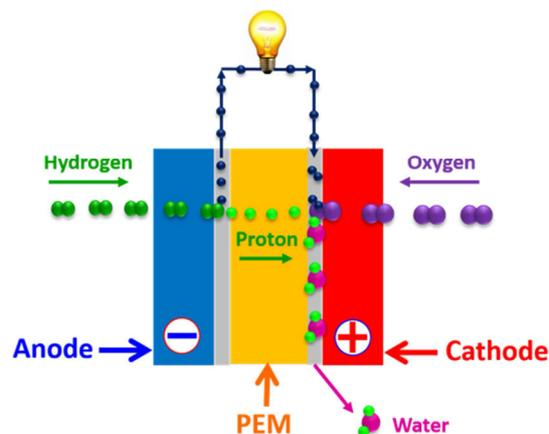
**Figure 1.1.** Schematic diagram of a single PEMFC.
