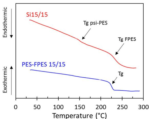
**Figure 3.** DSC curves of PES-FPES 15/15 and Si15/15 membranes.
