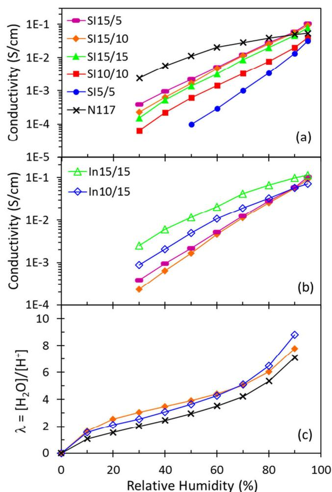
**Figure 11.** Proton conductivity as a function of relative humidity of SiX/Y ionomers in comparison with (a) Nafion<sup>®</sup> 117, and (b) InX/Y ionomers. (c) Water uptake as a function of relative humidity of SiX/Y ionomers in comparison with InX/Y ionomers.
