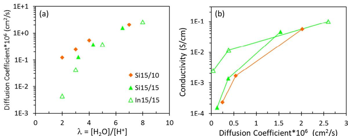
**Figure 12.** (a) Diffusion coefficient at low hydration number and (b) proton conductivity as a function of diffusion coefficient of SiX/Y ionomers in comparison to InX/Y ionomer.
