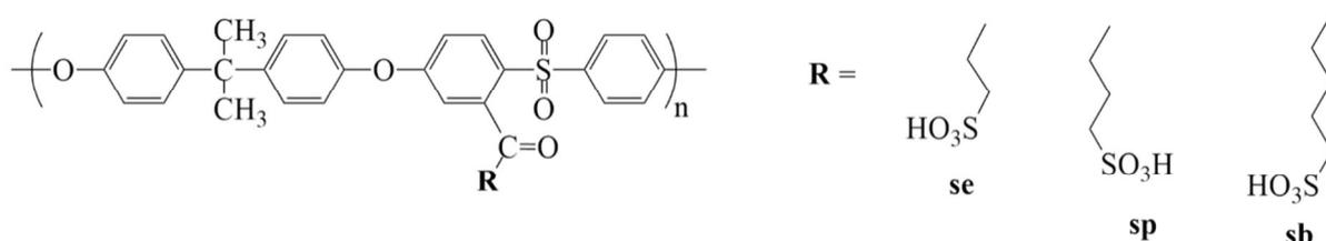
**Figure 3.18.** PESa bearing different sulfoalkyl side chains.
