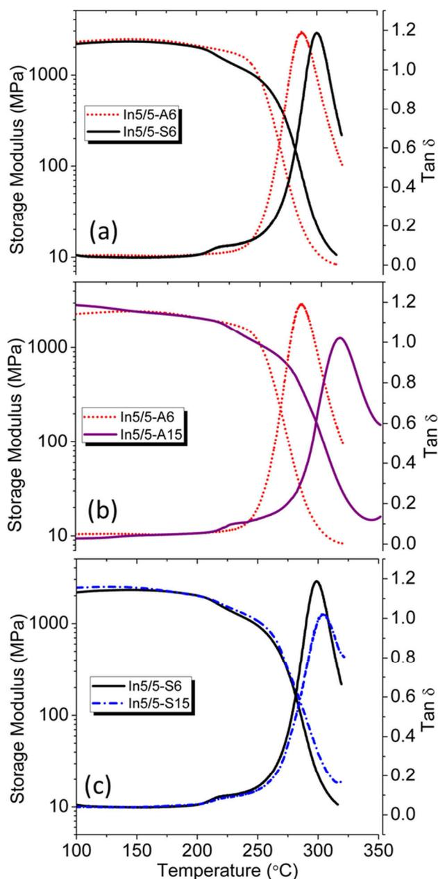
**Figure 6.** DMA profiles of In5/5 membranes in lithium-salt form: Storage modulus and  $\tan \delta$  vs temperature. (a) Membranes cast from DMAc and DMSO at 60 °C. (b) Membranes cast from DMAc at 60 °C and annealed at 150 °C (c) Membranes cast from DMSO at 60 °C and annealed at 150 °C. The membranes were washed in water and well dried before to perform DMA.
