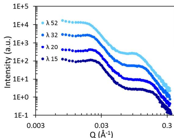
**Figure 6.** Incoherent background-subtracted SANS spectra of In5N10 membranes upon hydration degree. The spectra are shifted vertically for clarity.
