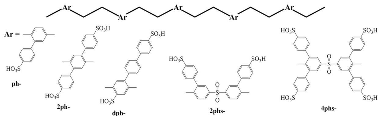
**Figure 3.14.** Representatives of aromatic ionomers bearing various phenylene side chains.
