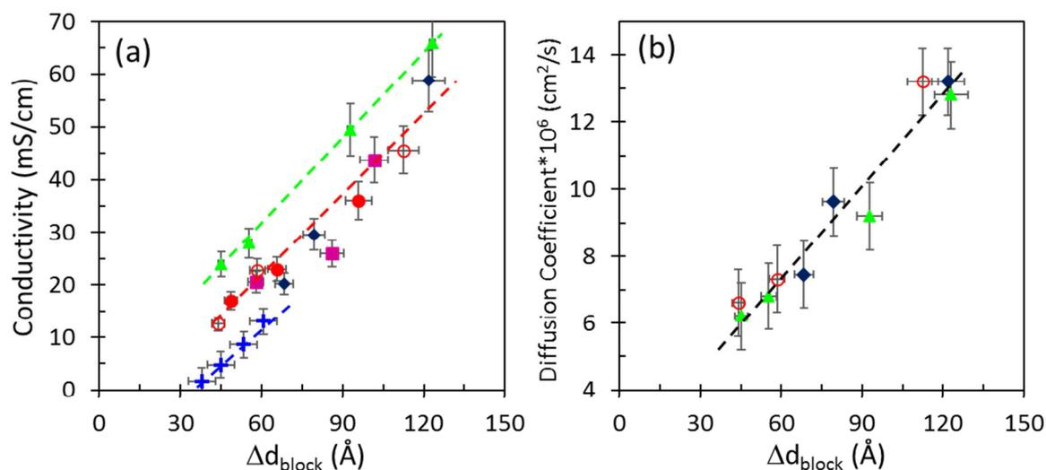
**Figure 9.** Variations of (a) the proton conductivity  $\sigma_i$  and (b) the water self-diffusion coefficient  $D_s$  as a function of the block structure expansion defined by  $\Delta d_{\text{block}}$ . In2.5/5 (blue +), In5/5-1 (red ●), In5/5-2 (red ○), In7.5/5 (green ▲), In10/10 (purple ■), In15/15 (dark blue ◆).
