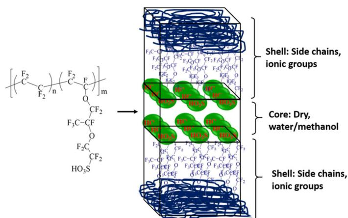
**Figure 2.3.** The sandwich-like model. Scheme adapted with permission from ref.<sup>42</sup> Copyright 2001 Elsevier.
