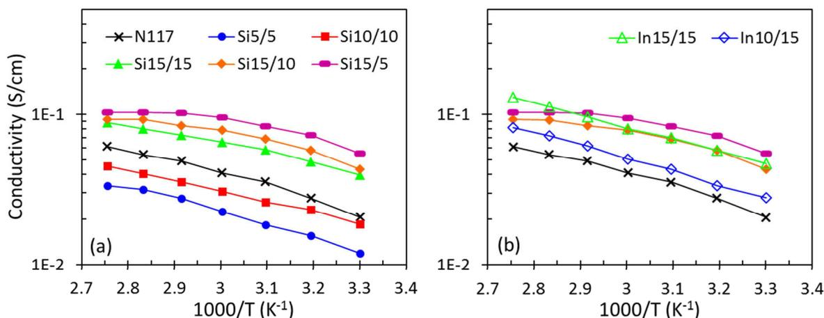
**Figure 9.** Proton conductivity of SiX/Y ionomers at 95 % RH as function of 1000/T; a) in comparison with Nafion<sup>®</sup> 117 and b) in comparison with InX/Y with similar IEC and water uptake, and Nafion<sup>®</sup> 117.
