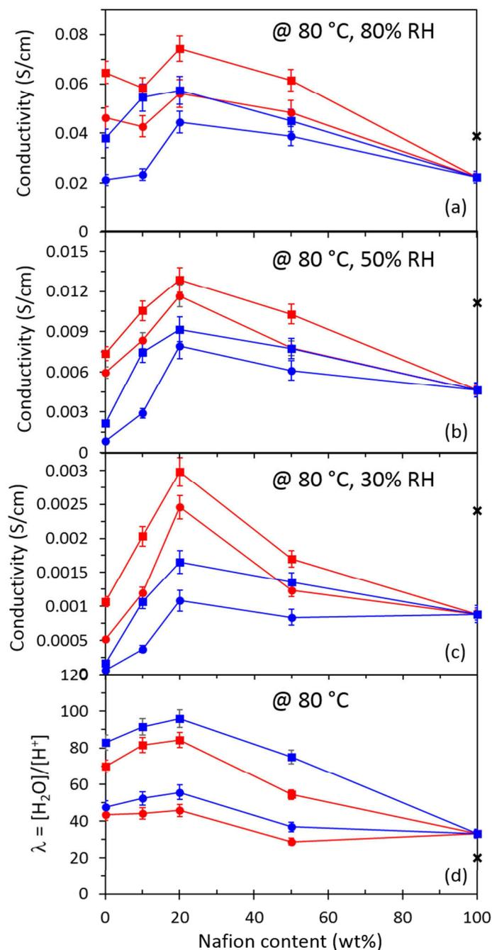
**Figure 4.** Proton conductivity at (a) 80% RH, (b) 50% RH, (c) 30% RH and (d) water uptake as a function of Nafion content in comparison with Nafion 117 (×) and cast Nafion. The pure InX/Y ionomer corresponds to 0 and pure Nafion to 100 on the x-axis. All the measurements were performed at 80 °C. In5/5N (blue ●), In5/5N-A (red ●), In10/10N (blue ■), In10/10N-A (red ■).
