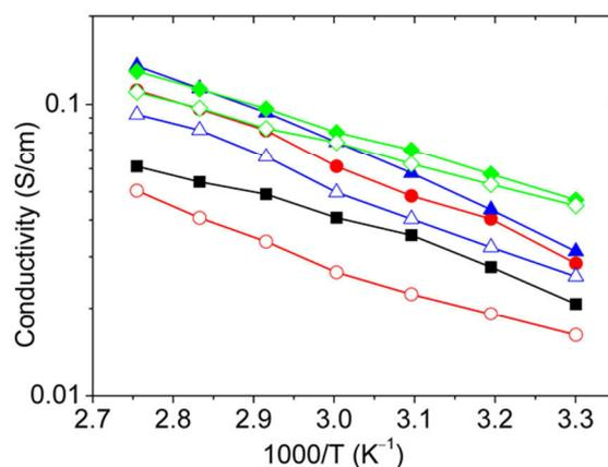
**Figure 10.** Evolution of proton conductivity with 1000/T at 95% of RH of InX/Y annealed membranes: In5/5-S15 (red ●), In10/10-S15 (blue ▲), In15/15-S15 (green ◆), In5/5-A15 (red ○), In10/10-A15 (blue Δ), In15/15-A15 (green ◇), Nafion 117 (black ■). (Errors limits for conductivities are ±14%).
