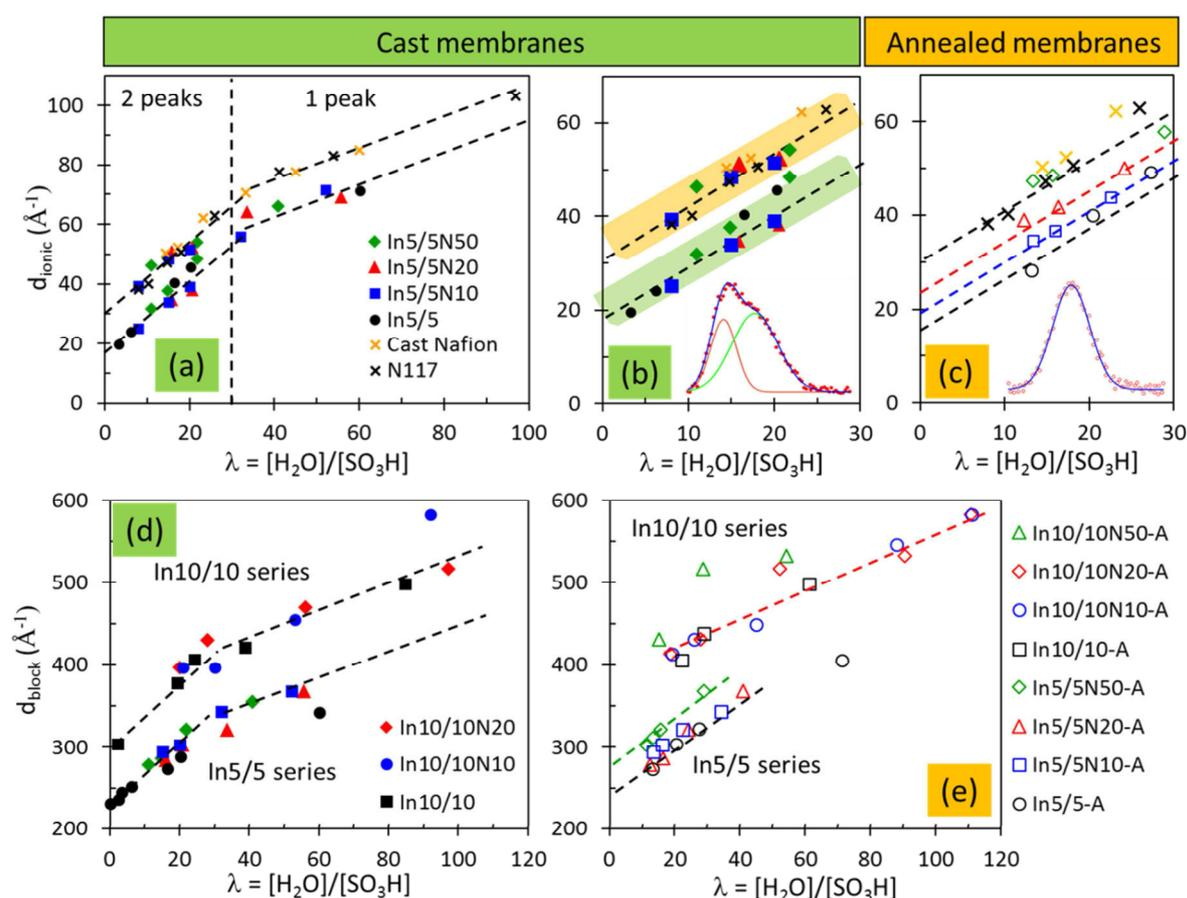
**Figure 7.** Variations of the ionic (top) and block (bottom) correlation distances of cast (a, b, d) and annealed (c, e) membranes upon  $\lambda$ . The cast Nafion, commercial Nafion and InX/Y ionomer ionic domain dilution laws are plotted for comparison.
