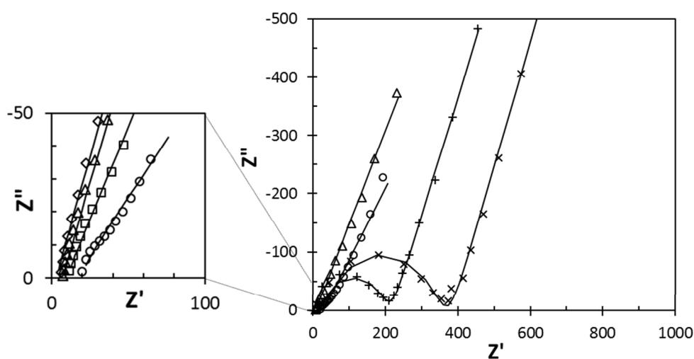
**Figure S3.** Nyquist plots of In5/5-2 at different hydration numbers (symbols) and corresponding fitted curves (lines).  $\lambda = 5$  ( $\times$ ),  $\lambda = 6$  ( $+$ ),  $\lambda = 17$  ( $\circ$ ),  $\lambda = 20$  ( $\square$ ),  $\lambda = 37$  ( $\triangle$ ),  $\lambda = 60$  ( $\diamond$ ). Some overlapped curves were removed for clarity.
