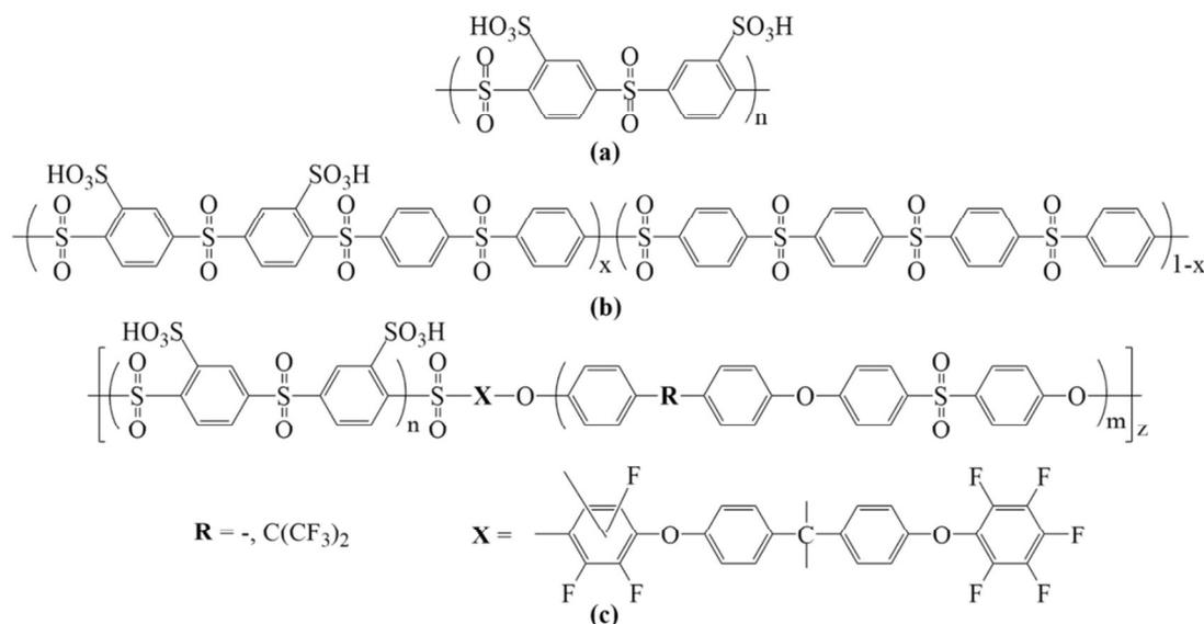
**Figure 3.5.** Chemical structure of (a) homopolymer as-PPS100, (b) random ionomer as-PPS<sub>x</sub>, (c) block copolymer as-PPS/PES (R = -) and as-PPS/6FPES (R = C(CF<sub>3</sub>)<sub>2</sub>).
