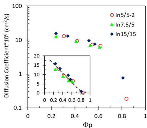
**Figure S7.** Water self-diffusion coefficient vs polymer volume fraction ( $\phi_p$ )
