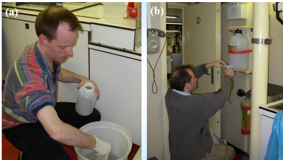
Figure 2.6. Mixing methods for subsampling of seawater for filtration: (a) seawater is stirred up with a measuring cylinder and then subsampled using a 1L container, (b) seawater is mixed by gently tumbling a closed 10 L container mounted on a rotating frame attached to the wall in the wet lab of the ship.
