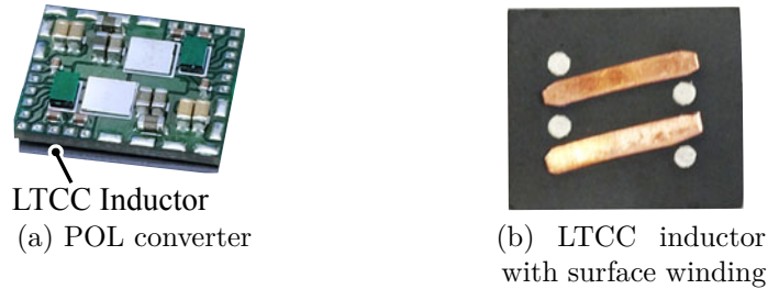
Figure 1.3.6: Integrated POL converter with LTCC inductor [51]
