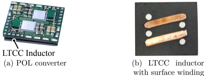
Figure 1.3.6: Integrated POL converter with LTCC inductor [51]
