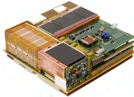
(b) 96.4 %, 8.18 kW/L interleaved full-bridge inverter [37]
