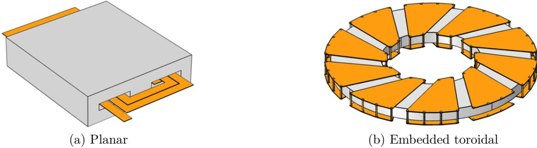
Figure 3.5.8: Inductor technologies
