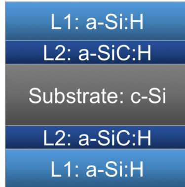
Figure 2.1: Schematic of a-Si:H heterostructure sample.
