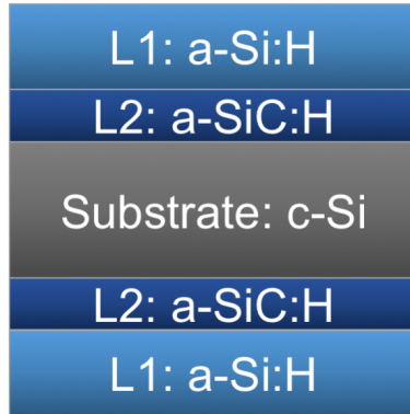
Figure 2.1: Schematic of a-Si:H heterostructure sample.
