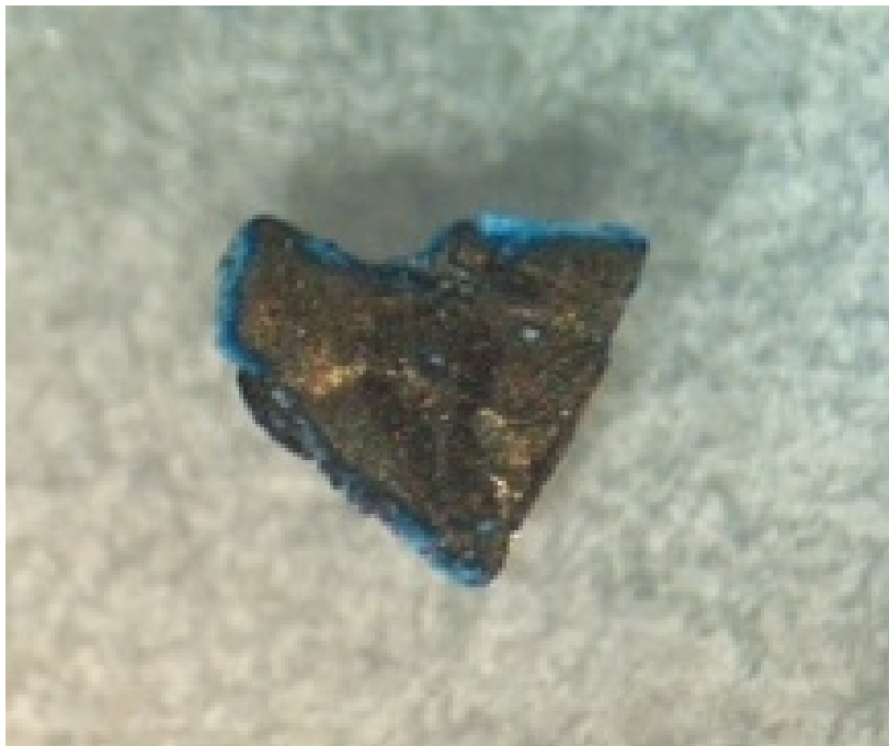
Figure III.6: (Left) \text{Ca}_2\text{CuO}_2\text{Cl}_2 crystal shows hydroxide damage after performing x-ray diffraction for two hours, using a cryojet to protect the crystal.
