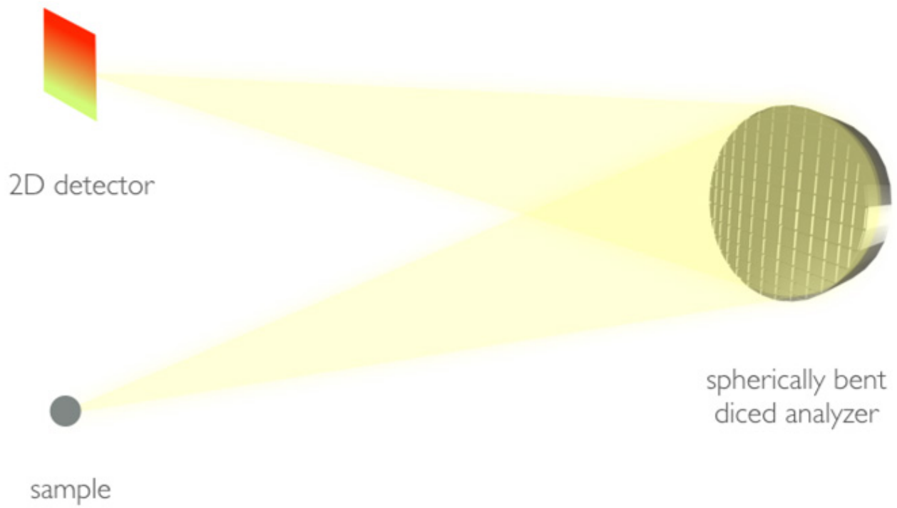
Figure 1: Schematic of the high resolution RIXS setup. The scattered x-ray beam is reflected by a 100 mm diameter spherically bent 'diced' crystal analyzer. The analyzer filters, disperses and focuses the x-ray photons on to a 2D pixelated detector
