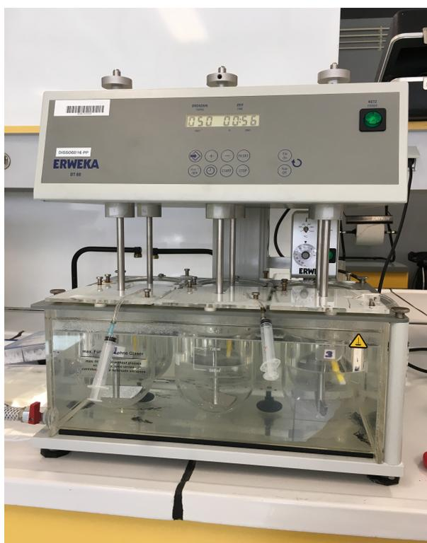
*Figure 42. A dissolution tester DT 60 (type II dissolution apparatus)*
