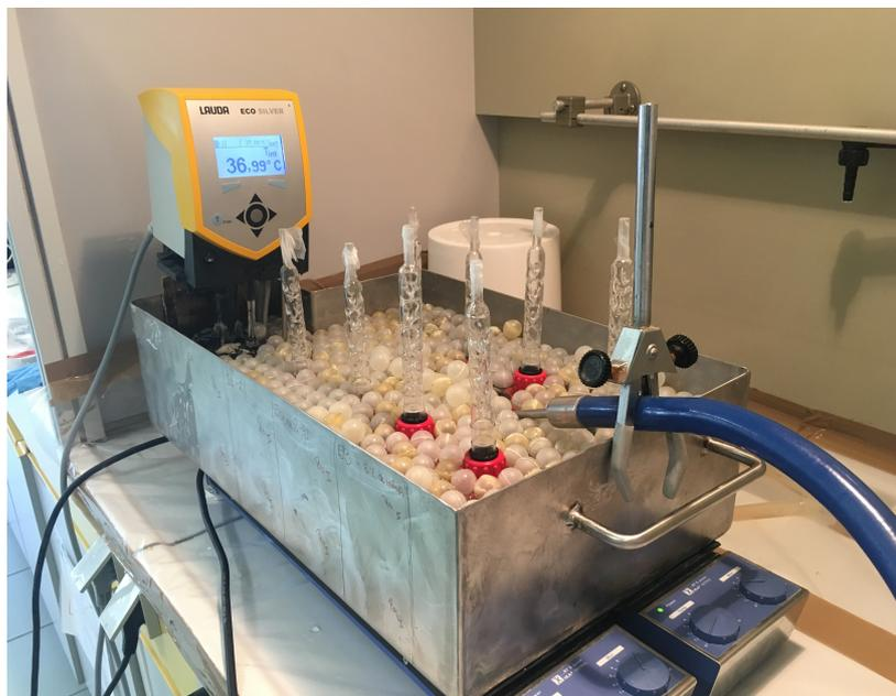
*Figure 31. Experimental apparatus for solubility tests (37°C)*
