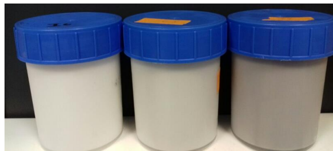
Fig. 2-14 Photograph of liquid tissue-simulating phantoms.
