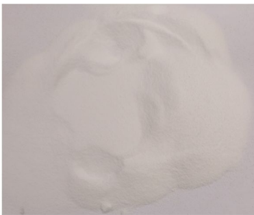
Cat. I: Not caked/very soft cake disintegrated to powder or small brittle crumbles when demolded
