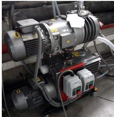
FIGURE 7.2: The roughing pump is a combination of an E2M80 rotary pump with an EH250 mechanical booster (both from Edwards Vacuum Ltd), yielding a pumping speed of 274 \text{ m}^3/\text{h} .
