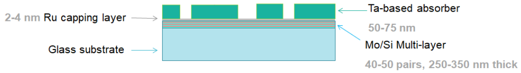
FIGURE 4.1: Schematic representation of Ta-based EUV photomasks. Adapted from [4].
