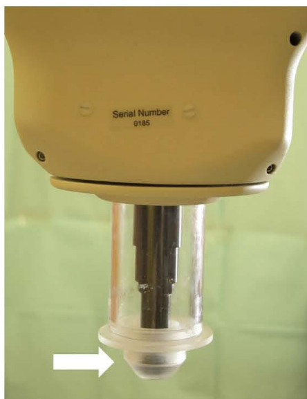
Fig. 2 Vivascope adaptor for the ocular surface. Adapted tip (arrow) for the ophthalmic application of Vivascope 1500.
