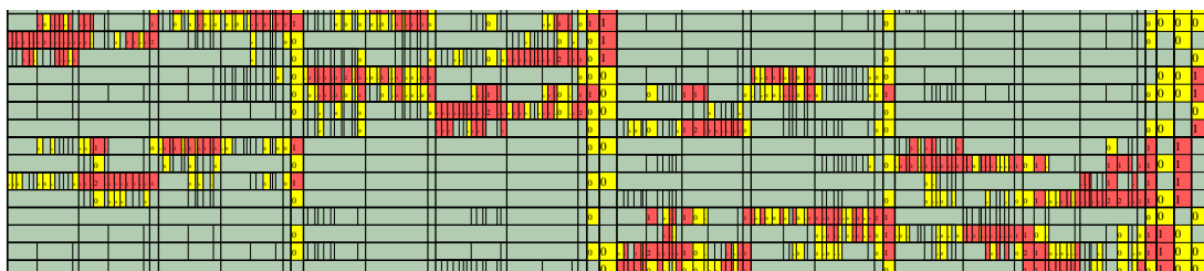
Figure B.6: Example of BEM-FEM matrix A_{sv} storage using Scotch ND+ for the FEM mesh in a FEM/BEM coupling with 8000 unknowns.
