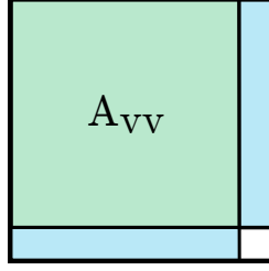
Figure 1.44: Structure of the assembled matrix Y used to compute each Schur complement in the Multi-Factorization routine.
