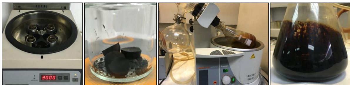
Figure 3-1 Asphaltenes centrifugation and drying, and malthenes recovery
