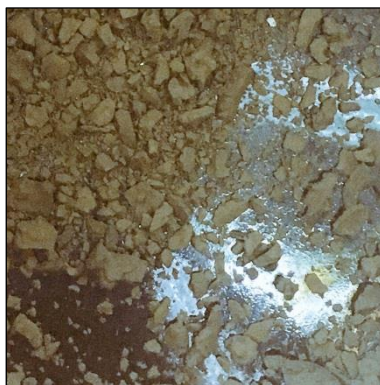
Figure 3-2 Asphaltenes and malthenes for bitumen recombination
