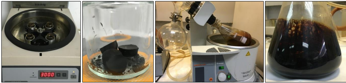
Figure 3-1 Asphaltenes centrifugation and drying, and malthenes recovery
