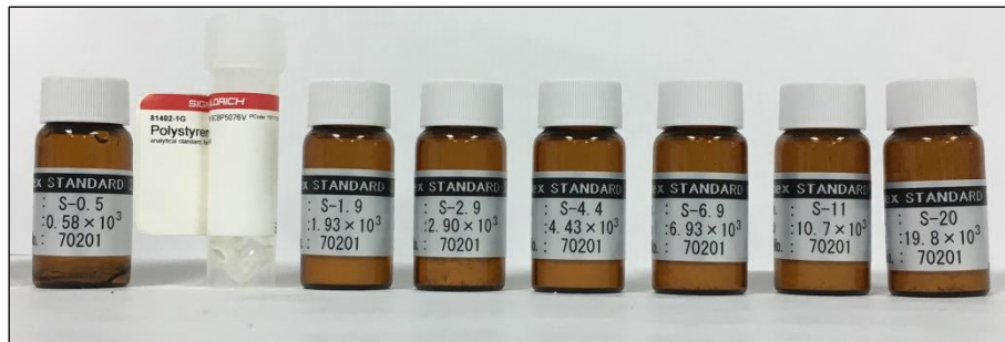
Figure 3-8 GPC standards for curve calibration
