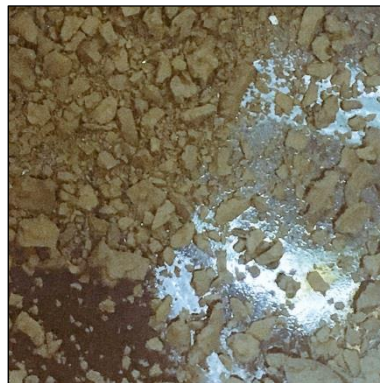
Figure 3-2 Asphaltenes and malthenes for bitumen recombination
