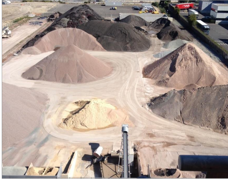
Figure 2-2 Aggregates for asphalt mixture manufacture
