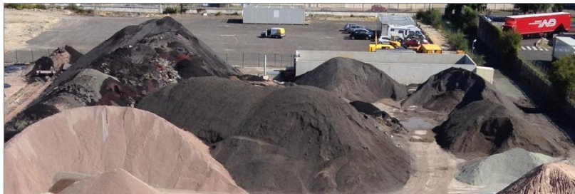
Figure 2-11 RAP stockpile ready to be use on mixture manufacture
