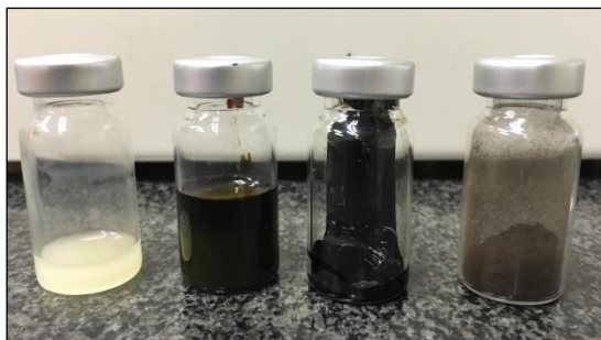
Figure 2-15 SARA fractions, Saturates, Aromatics, Resins and Asphaltenes
